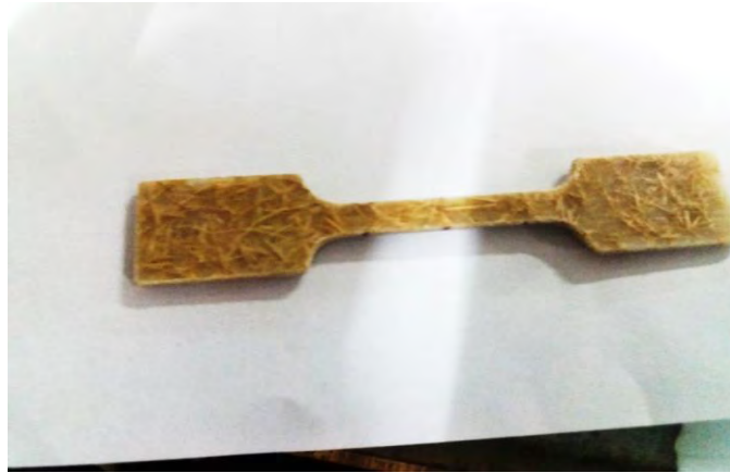
Figure 3.7: Photograph of a tensile test specimen
