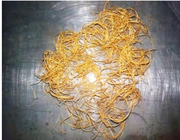
Figure 3.5: Alkali treated betel nut fiber
