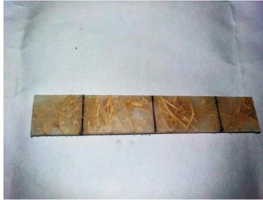
Figure 3.9: Photograph of a flexure test specimen
