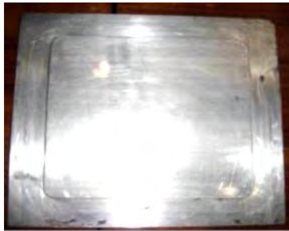
Figure 3.6: Die used for composite manufacturing
