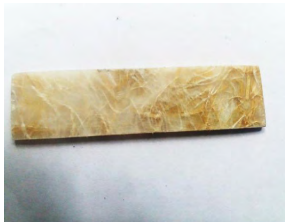
Figure 3.11: Impact test specimen
