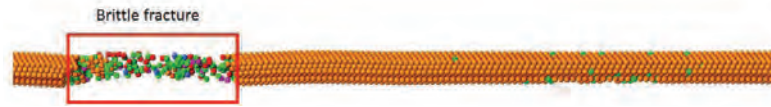
FIGURE 3.10: Atomistic configurations of nanowire of 2 nm diameter at 300 K for loading at \langle 111 \rangle direction during uniaxial tensile test.
