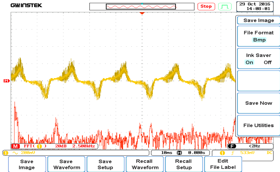
Figure 6.27: Input Current (Yellow) and its Fourier Transform (Red) for Modified-2 Single Phase Ćuk Rectifier for D = 0.5 From Oscilloscope
