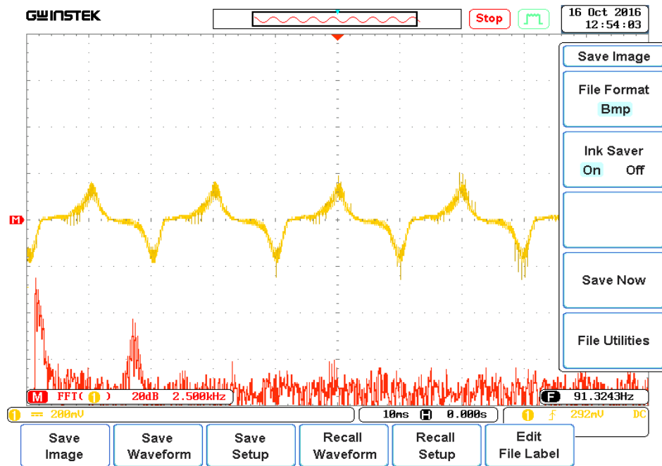
Figure 6.8: Output and Intermediate Capacitor Voltages (Red) for Modified-1 Single Phase Ćuk Rectifier of D = 0.5 From Oscilloscope
