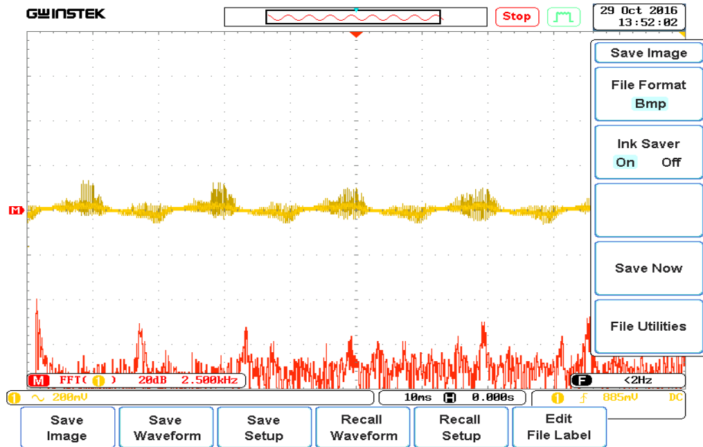
Figure 6.21: Input Current (Yellow) and its Fourier Transform (Red) for Modified-2 Single Phase Ćuk Rectifier for D = 0.3 From Oscilloscope
