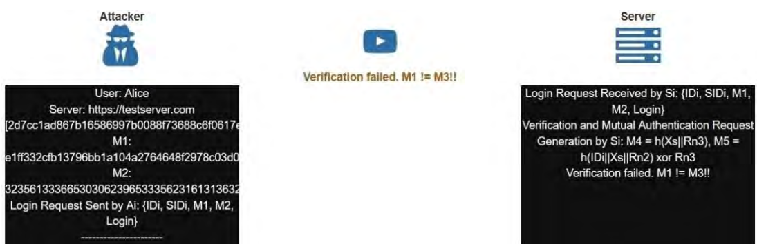
Fig. 7.16. Simulation of replay attack which involves the attacker and the server
