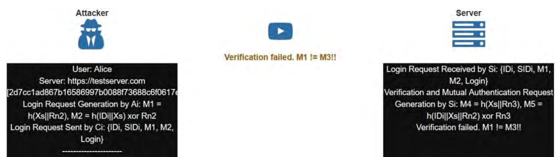
Fig. 7.14. Simulation of user impersonation attack which involves the attacker and the server
