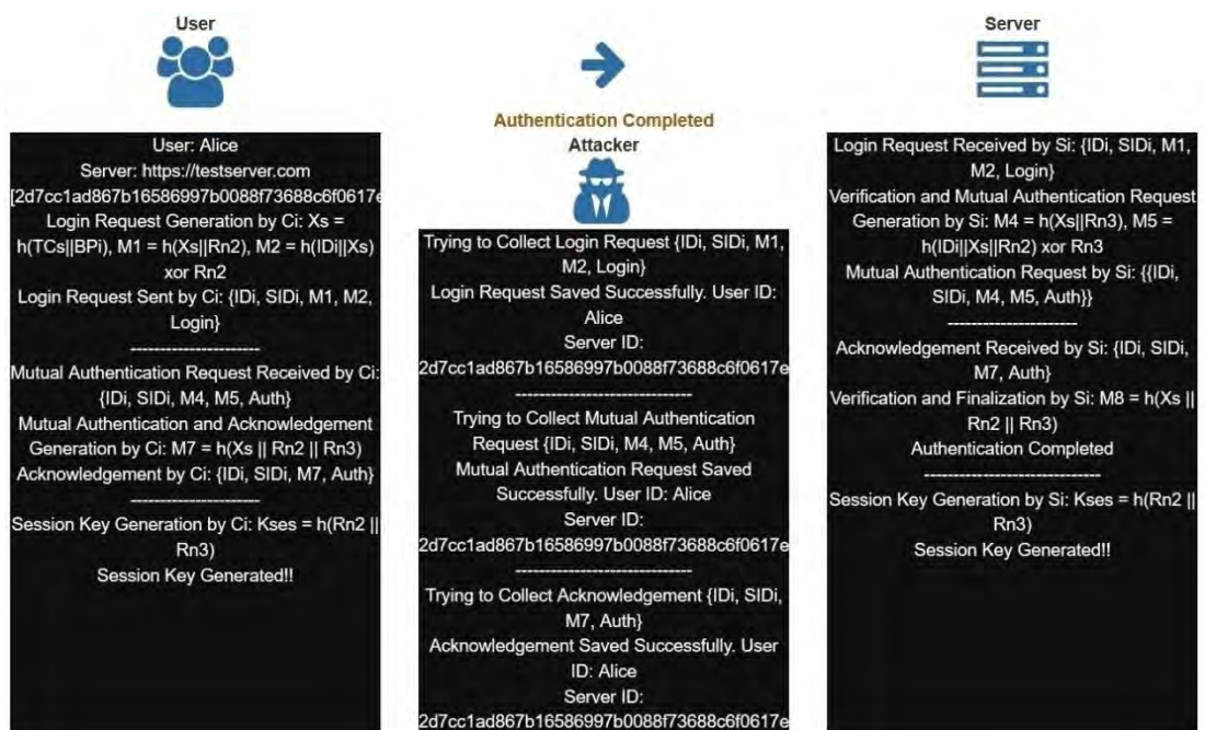
Fig. 7.5. Simulation of login and authentication phase which involves the user and the server
