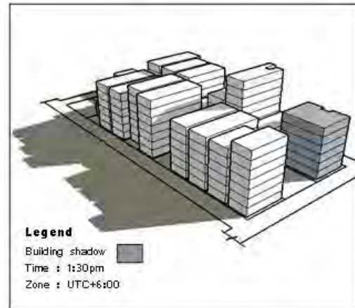
Fig 4.27 : Higher plot coverage and uniform height resulting into compact settlement causing blockage of sunlight, ventilation and view.
