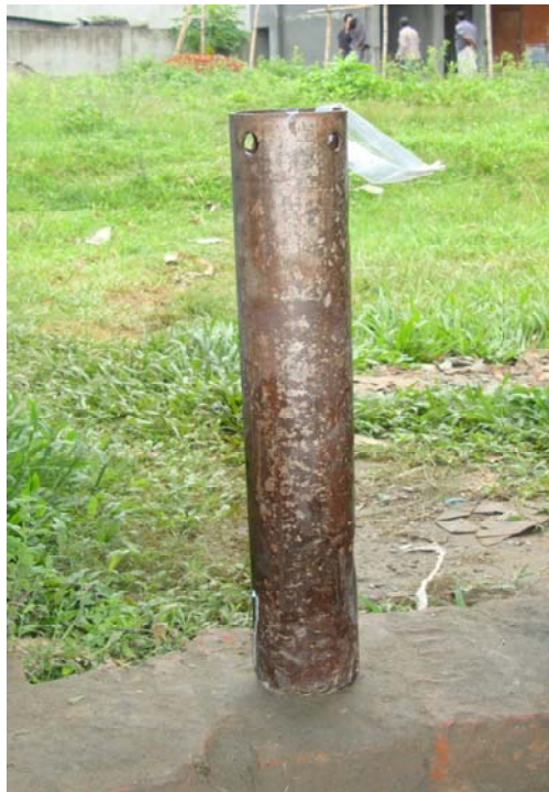
Figure 2.9: Schematic view of a Currently Practiced Shelby Tube Sampler
