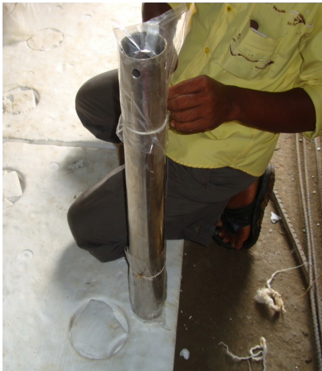
Fig. 3.5: Covering the sampler with plastic packet to make the sample airtight
