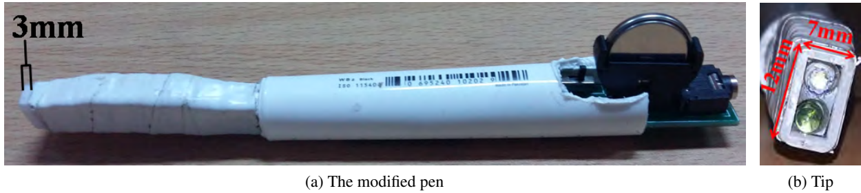
Figure 5.5: Modified pen with its tip
