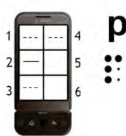
Figure 2.2: VBraille representation of a Braille character
