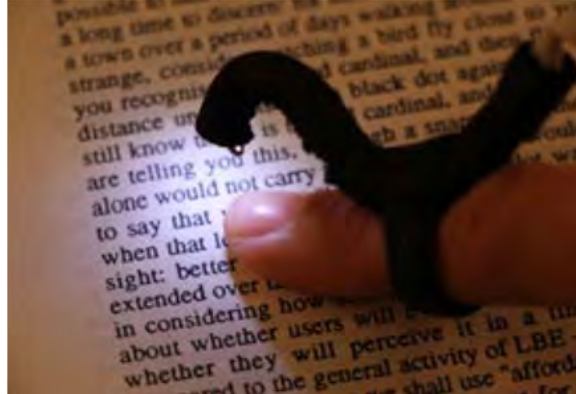
Figure 2.5: Finger-mounted camera in HandSight
