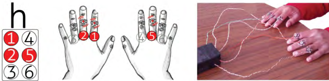
Figure 2.7: UbiBraille - Braille-reading vibrotactile prototype
