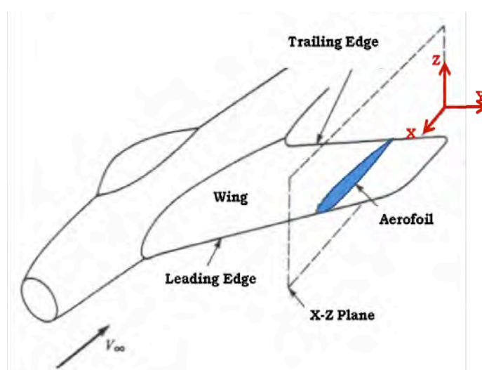
Figure 3.1: Wing and Aerofoil with Nomenclature [29]
