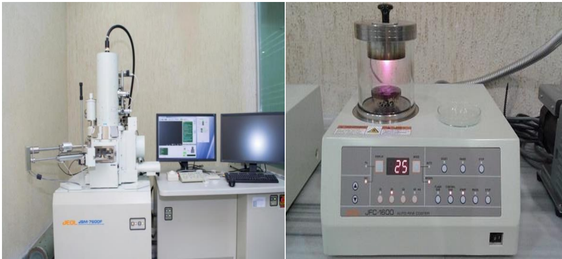
Fig. 3.10 FESEM instruments (Model: JEOL JSM 7600F) with an Auto Fine Coater (Model: JFC 1600).
