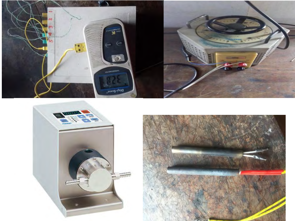
Figure 3.4: Thermocouple display and selector switch, variac, gear pump and the cartridge heater used in the experiment
