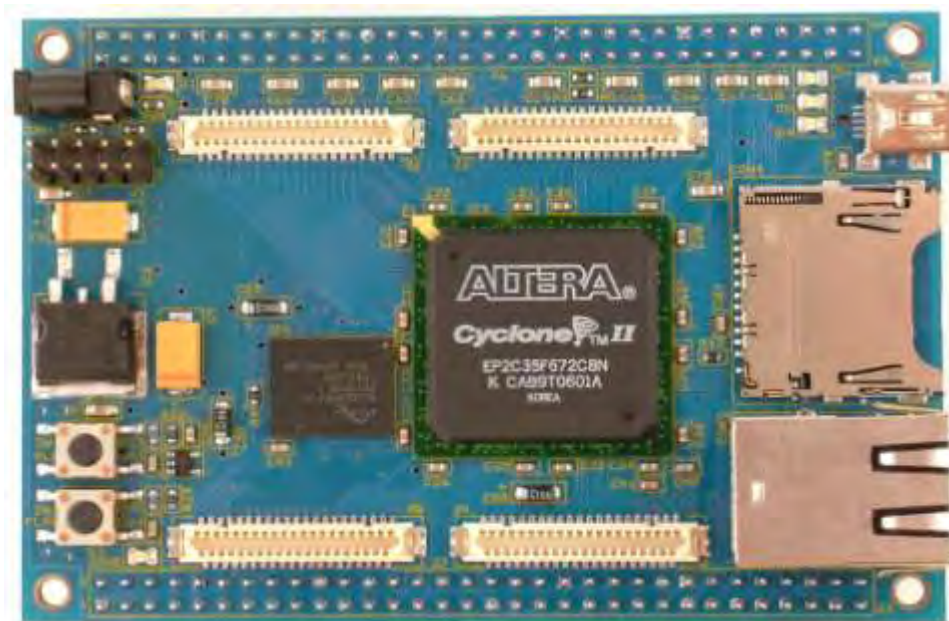
Figure 2.11 An Altera Cyclone II FPGA (DE2 Board)
