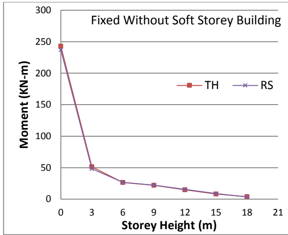
Figure 4.33: Corner Column Moment (TH vs RS) for Fixed Base without Soft Storey Building
