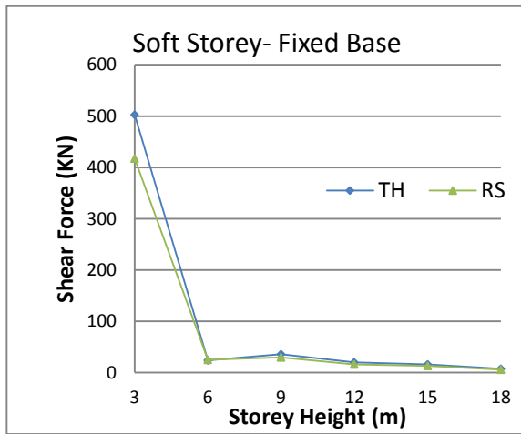
Figure 4.60: Interior Column Shear (TH Vs RS) for Soft Storey Fixed base building
