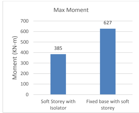
Figure 4.15: Corner Column Moments for Soft Storey Building for assign Time History
