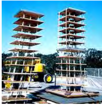
Figure 2.2: Snapshot of shake-table testing of a base-isolated (right) and a regular (left) building model
