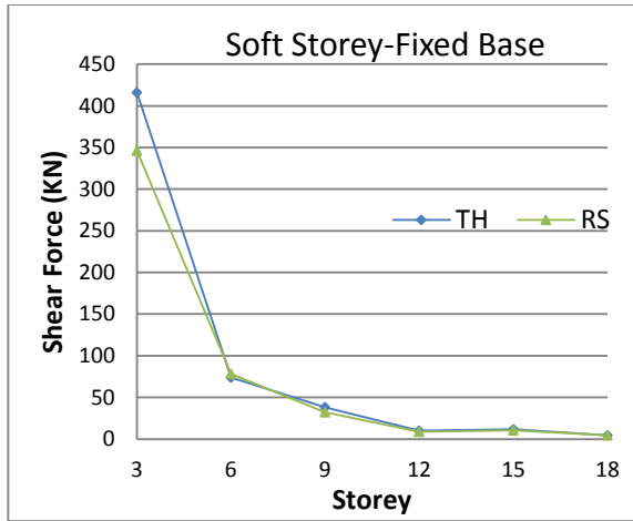
Figure 4.62: Corner Column Shear (TH Vs RS) for Soft Storey Fixed base building
