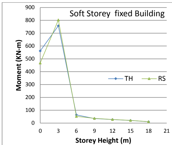
Figure 4.34: Interior Column Moment (TH vs RS) for Fixed Base Soft Storey Building
