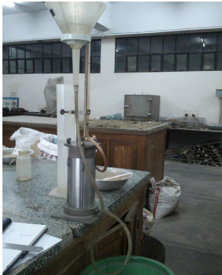
Fig. 3. 3 Photograph showing the set-up for falling head test.
