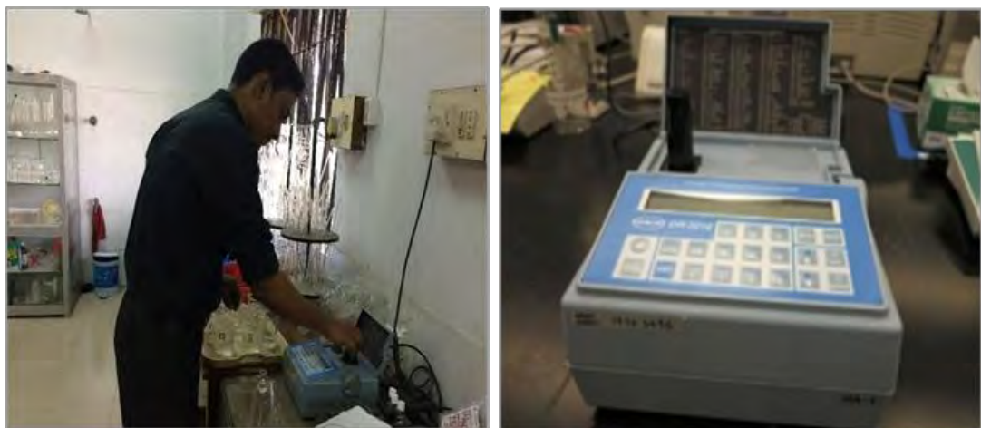
Figure 3.8: Measuring COD in HACH DR-2010 spectrophotometer.
