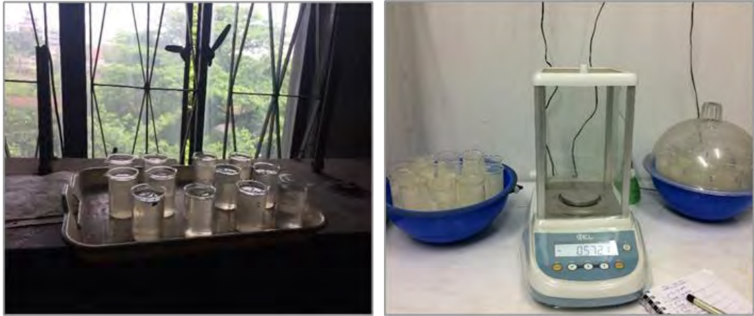
Figure 3.7: TDS beakers with water samples before drying in the oven (left) and cooling TDS beakers before weighing (right).
