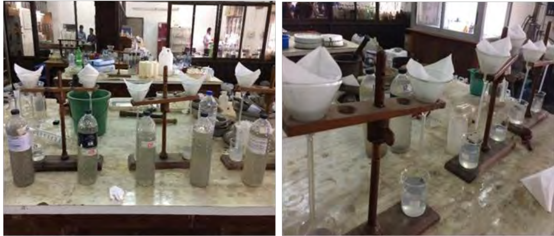
Figure 3.5: Filtering of river water samples
