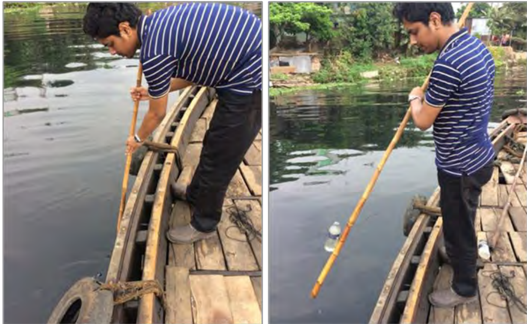
Figure 3.3: Collecting river water samples
