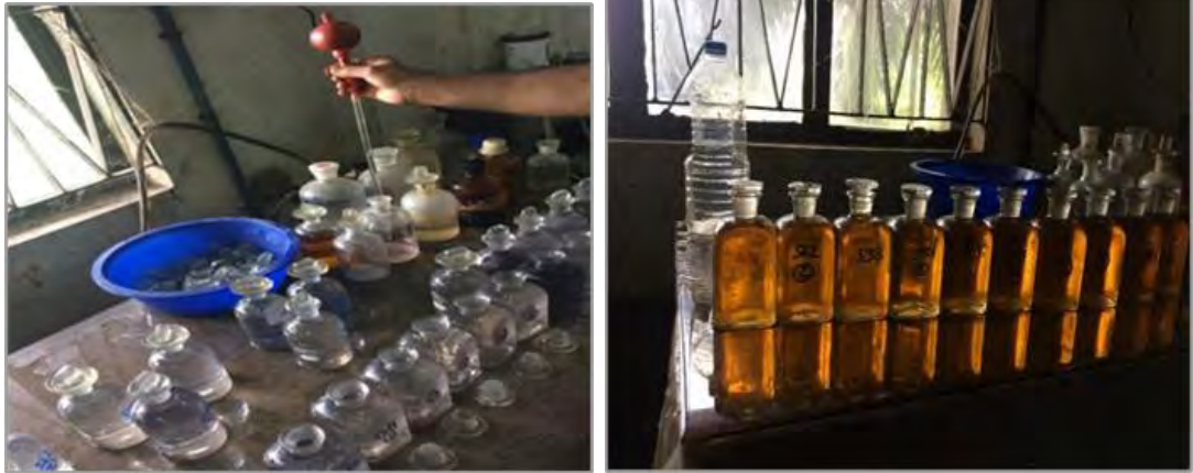
Figure 3.9: Preparing BOD bottles for DO measurement.
