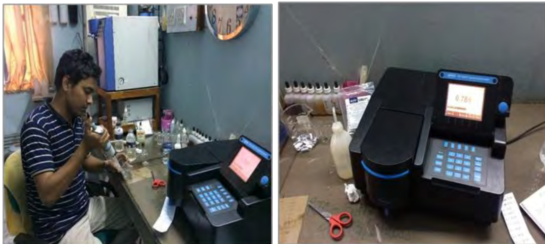
Figure 3.6: Measurement of ion concentrations ( \text{NH}_3^- , \text{NO}_3^- , and \text{PO}_4^{3-} ) in HACH DR-4000U spectrophotometer.
