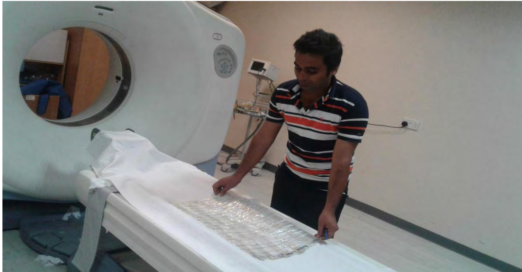
Figure 4.4: Placement of the TLD containing sheet on patient's bed just before starting of the scanning procedure
