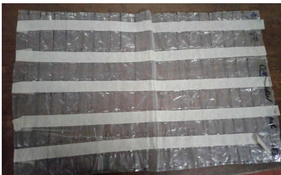
Figure. 4.3: Arrangement of TL chips between two polythene sheets
