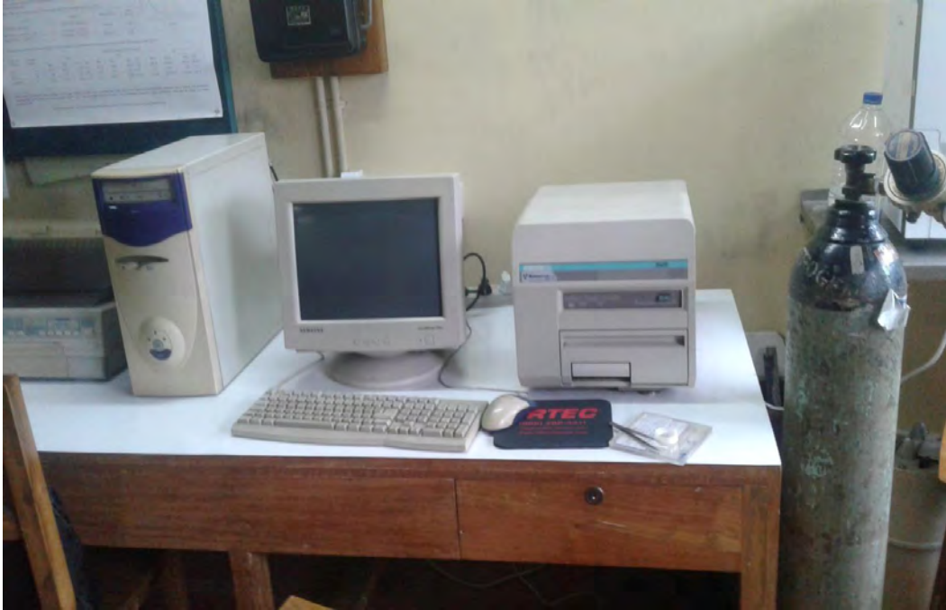
Figure 4.2: Harshaw TLD reader (Model 3500) set up for dose measurement
