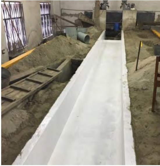
Figure 5.3: New rectangular main channel
