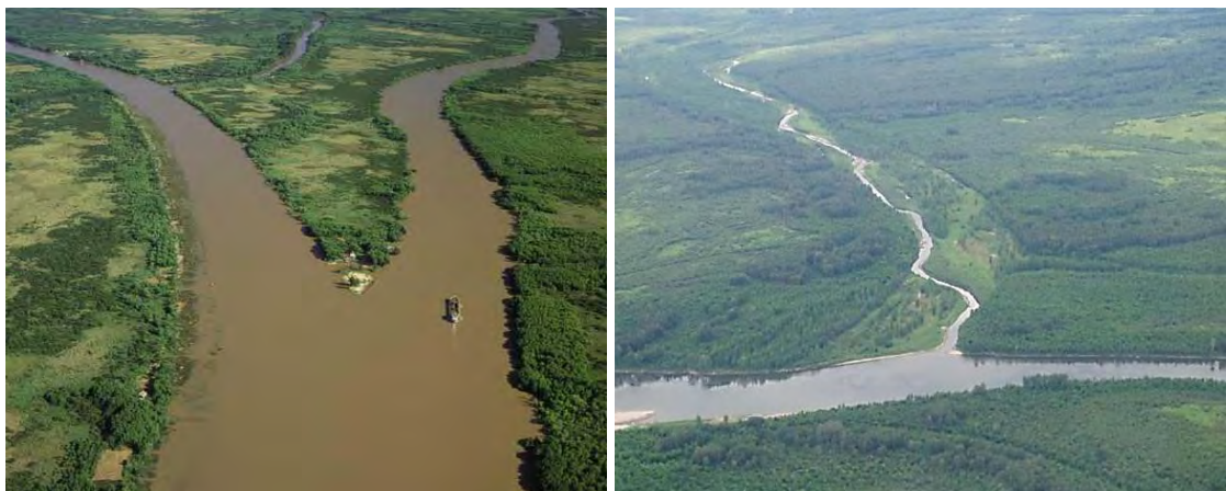
Figure 2.2: Difference between river bifurcation (left) and river offtake (right).
