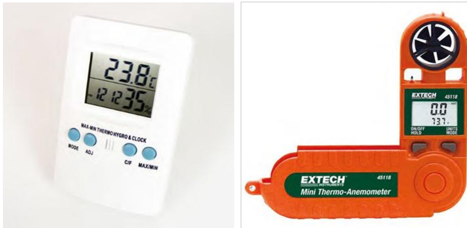
Fig 3.10 & 3.11: Image of Digital Thermometer Hygrometer (Zeal PH1000) and Image of Mini Thermo Anemometer (Extech 45118)
