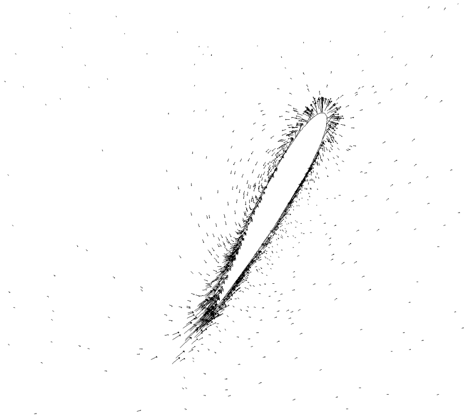
Fig. 6.55(e): Velocity vector of 6 Bladed Double layered Staggered H – Rotor VAWT; Solidity 1.5, \lambda=3.0 (inner layer blades at 240 degree)
