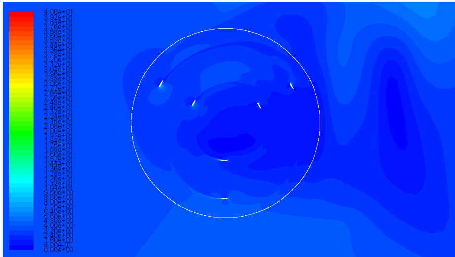
Fig. 6.30: Velocity contour of 6 Bladed Double layered H – Rotor VAWT; Solidity 0.75, \lambda=4.5 (60 degree)
