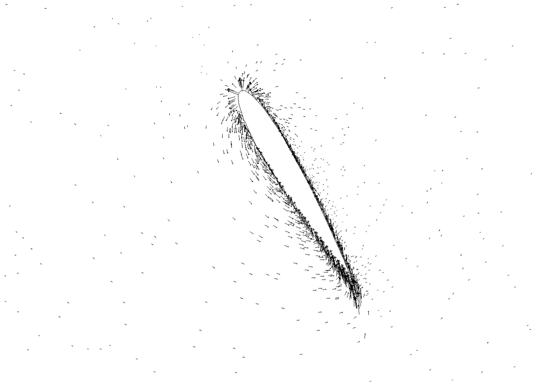
Fig. 6.55(f): Velocity vector of 6 Bladed Double layered Staggered H – Rotor VAWT; Solidity 1.5, \lambda=3.0 (inner layer blades at 300 degree)
