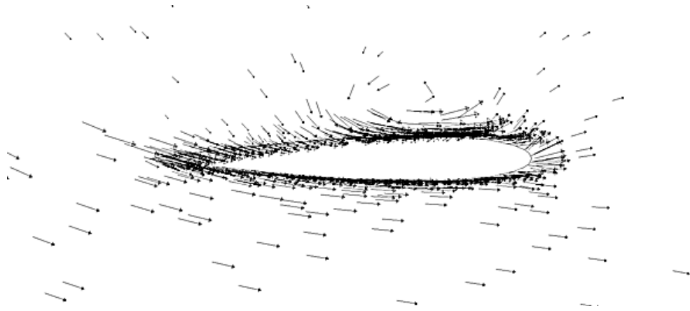
Fig. 6.16(d): Velocity vector of 3 Bladed Single layered H – Rotor VAWT; Solidity 1.0, \lambda=2.25 (blade at 180 degree)
