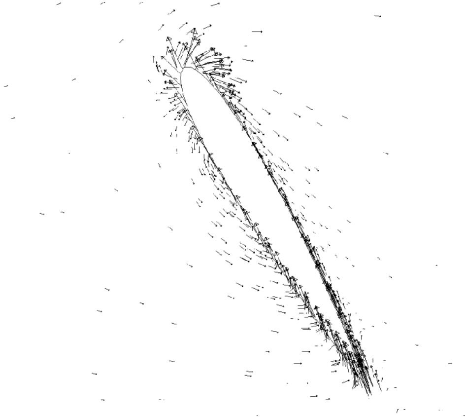
Fig. 6.15(f): Velocity vector of 3 Bladed Single layered H – Rotor VAWT; Solidity 0.7, \lambda=2.5 (blade at 300 degree)
