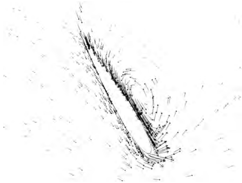
Fig. 6.36(c): Velocity vector of 6 Bladed Double layered H – Rotor VAWT; Solidity 0.75, \lambda=4.5 (inner layer blade at 120 degree)
