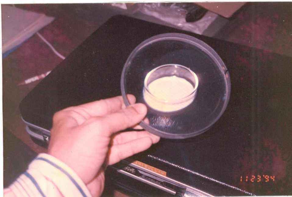
Plate B-7 : Membrane Filter (MF) Before Placing in Incubator.
