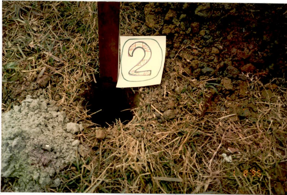
Plate B-9 : A Percolation Test Hole Showing Depth.
