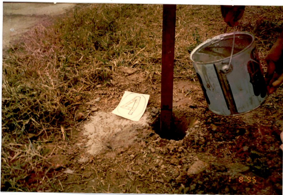
Plate B-10 : Septic Tank Effluent Being Poured in one of the Test Holes.
