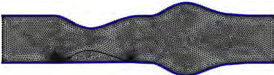
Figure 2.2c: Current mesh structure of elements for stenotic and aneurysmatic artery.
