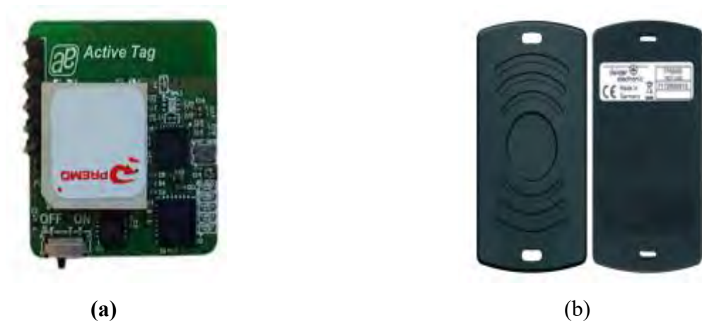
Figure 2.7: Example of (a) Active RFID tag and (b) Semi active RFID tag [48].
