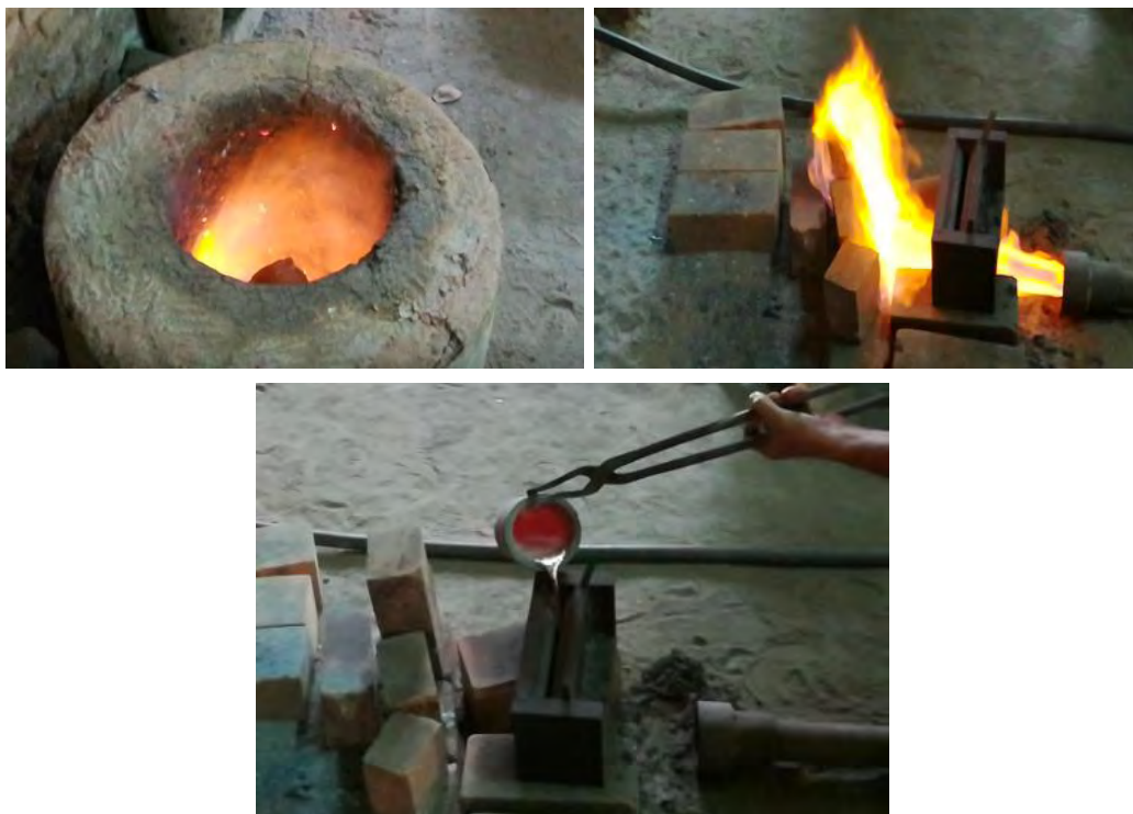
Figure 3.2 Melting of Zn-Sb in Pit Furnace
