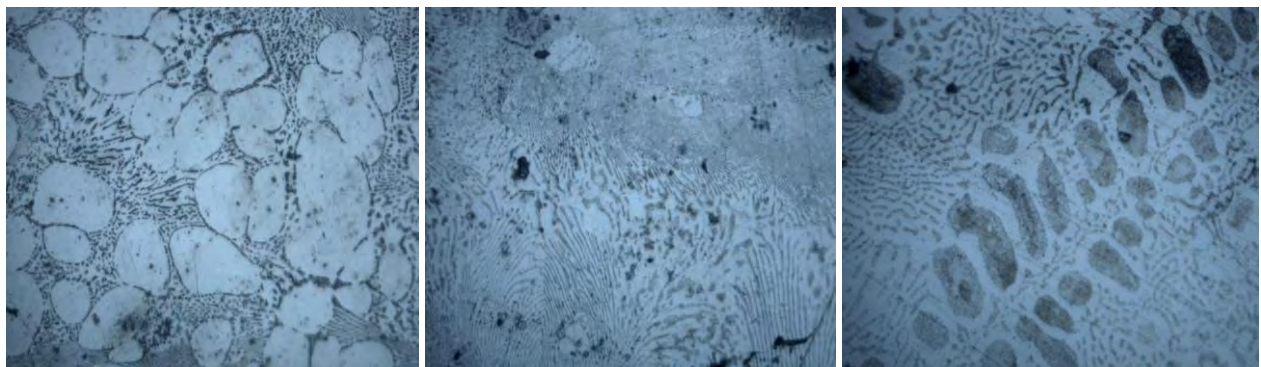
Figure 2. 13 Microstructure of Zn-0.3wt% Al, Zn-0.5wt% Al and Zn-0.7wt% Al respectively From this study, higher tensile stress and fracture strain were observed as the amount of Al was increased. Mechanical tests showed that the joint area was stronger than the parent material with
