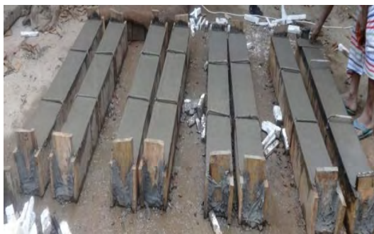
(e) Concrete specimens after casting
