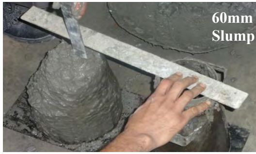
(a) Slump for column end zone concrete
