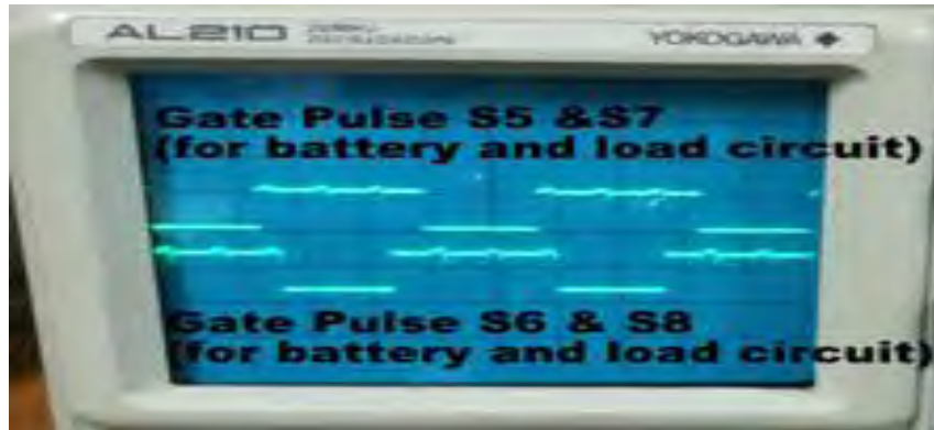
Figure 4.16: Gate Pulses for Battery and Load circuit
