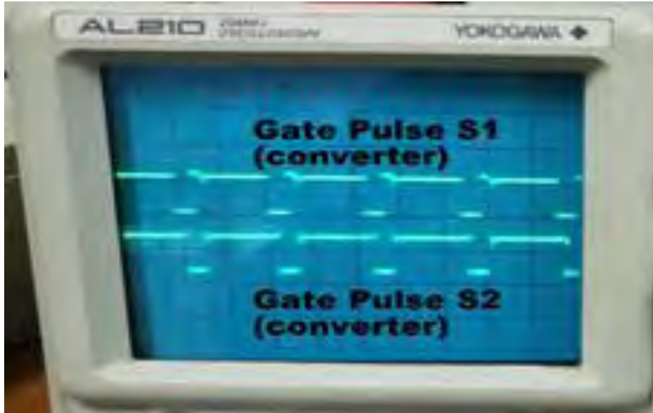
Figure 4.14: Gate Pulses for Isolated Flyback-Forward Converter
