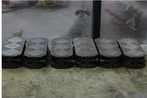
Figure 3.10: Mortar in molds after casting
