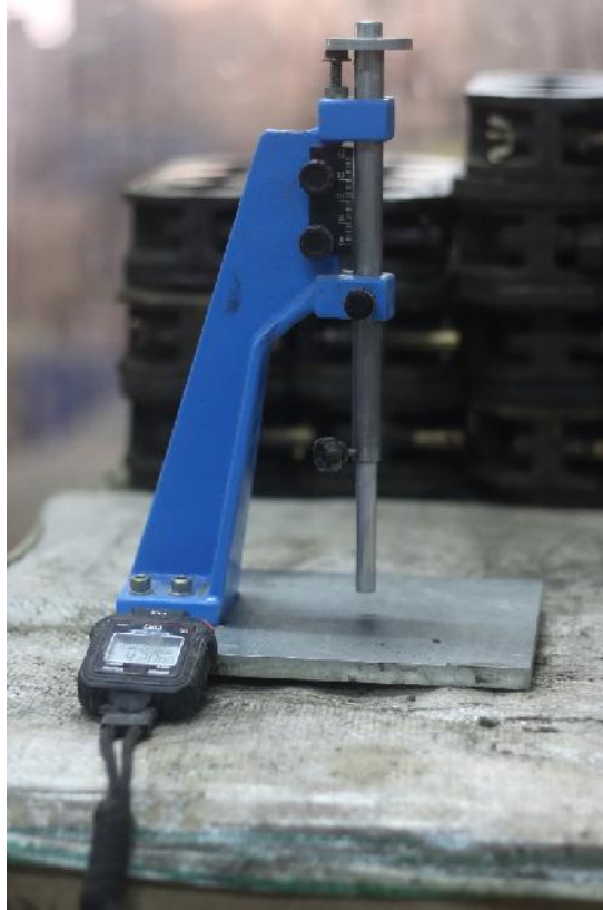
Figure 3.3: Vicat apparatus to determine normal consistency of cement
