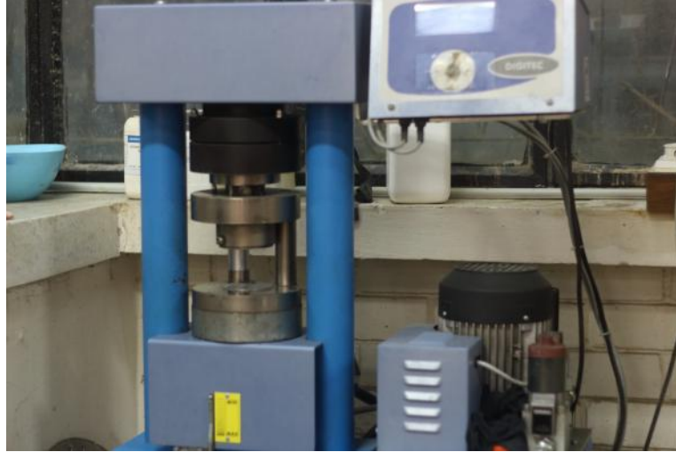
Figure 3.13: Cube in compression testing machine
