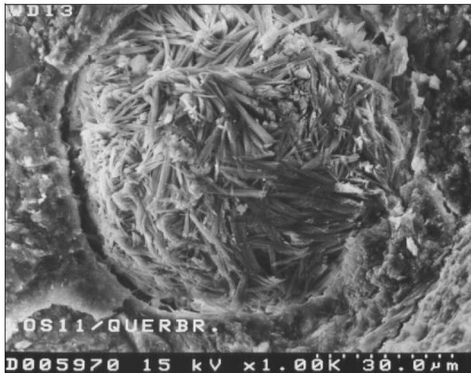
Figure 2.2: Air void completely filled with ettringite crystals (Stark and Bollmann, 1999)
