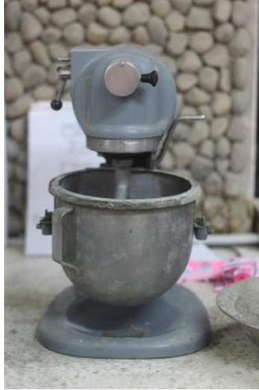
Figure 3.8: Mixer machine with bowl and paddle
