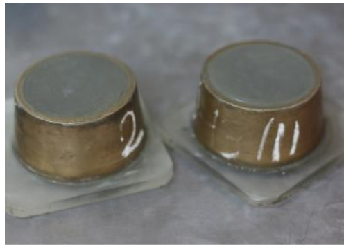
Figure 3.5: Setting time test molds
