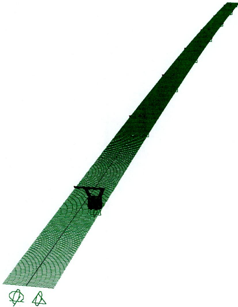
Fig. 5.16 3D View of the lateral prestressing tendon.
