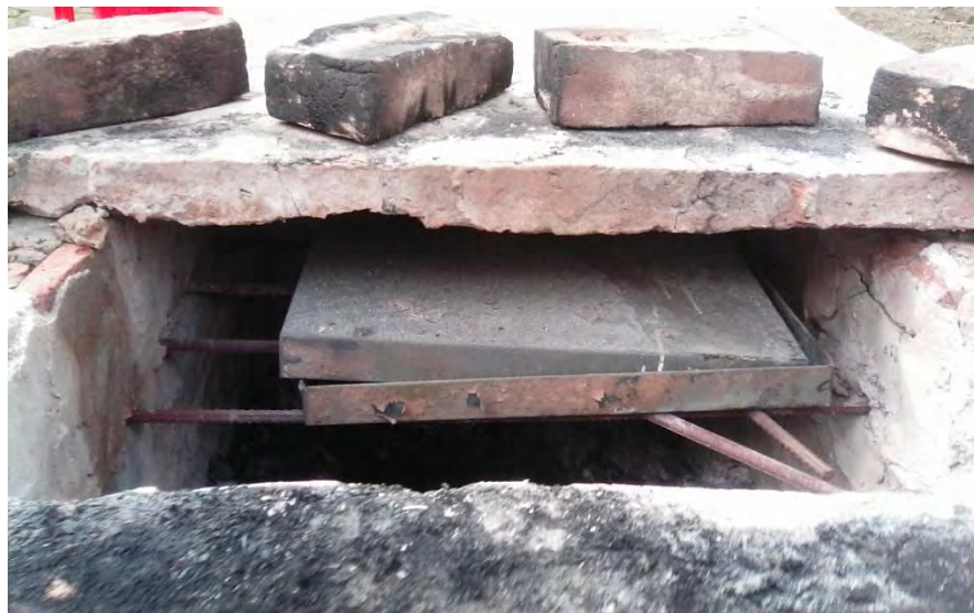
Figure A12 Sample placed in Brick furnace in covered condition
