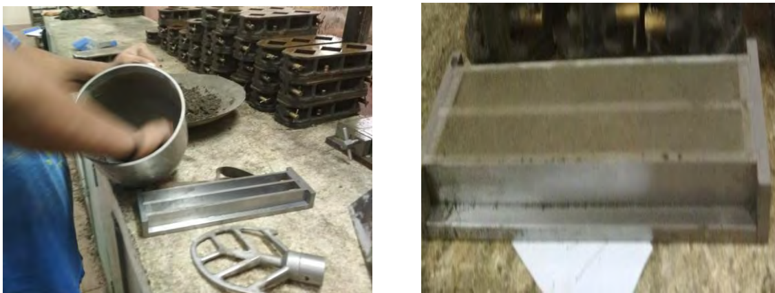
Figure 3.24: Molding of specimens for shrinkage test.
