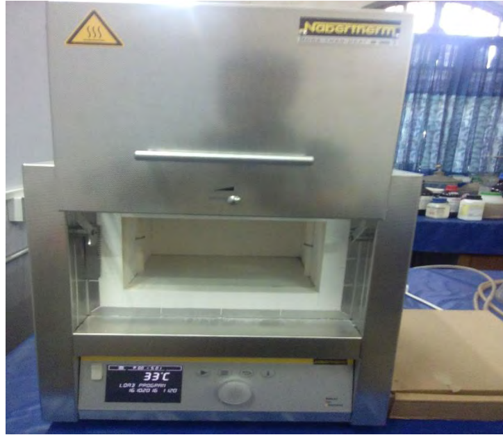
Figure A5 Muffle Furnace (maximum 1200 °C range)
