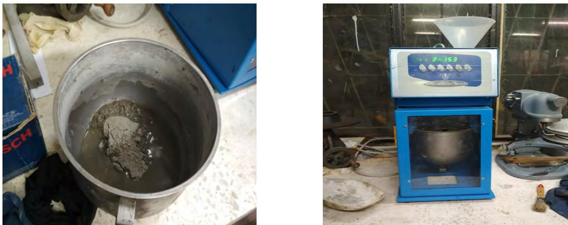
Figure 3.20: Automatic mortar mixer for proper mixing of ingredients
