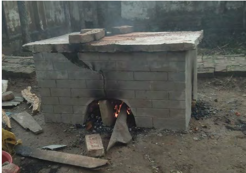
(b) Brick furnace during calcination
