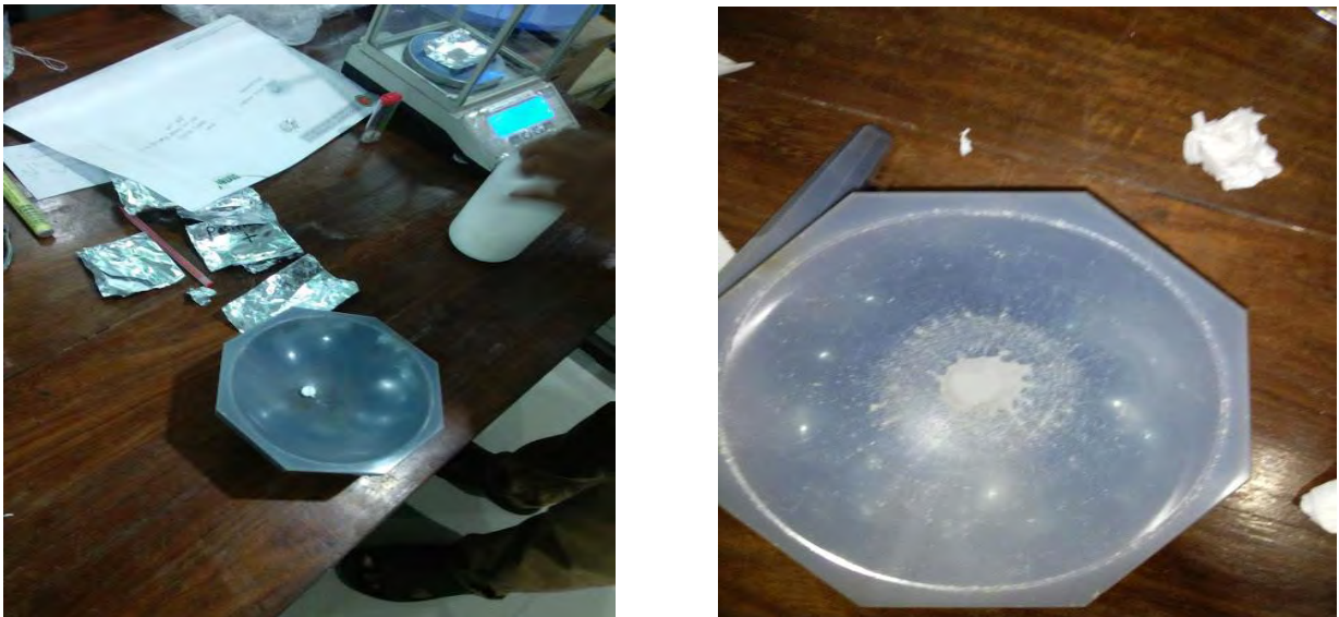
Figure 3.14: Binder mixing with bagasse ash
