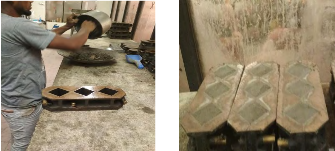
Figure 3.21: Molding of test specimens
