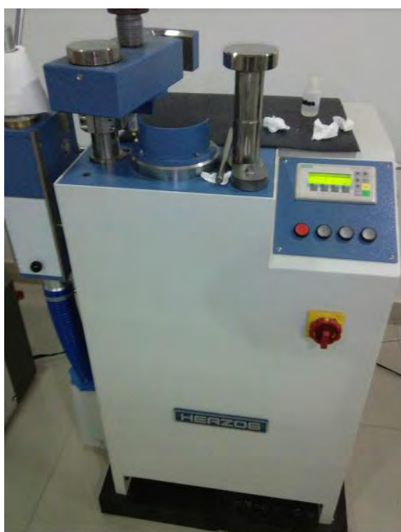
Figure A16 Press machine for XRF sample preparation
