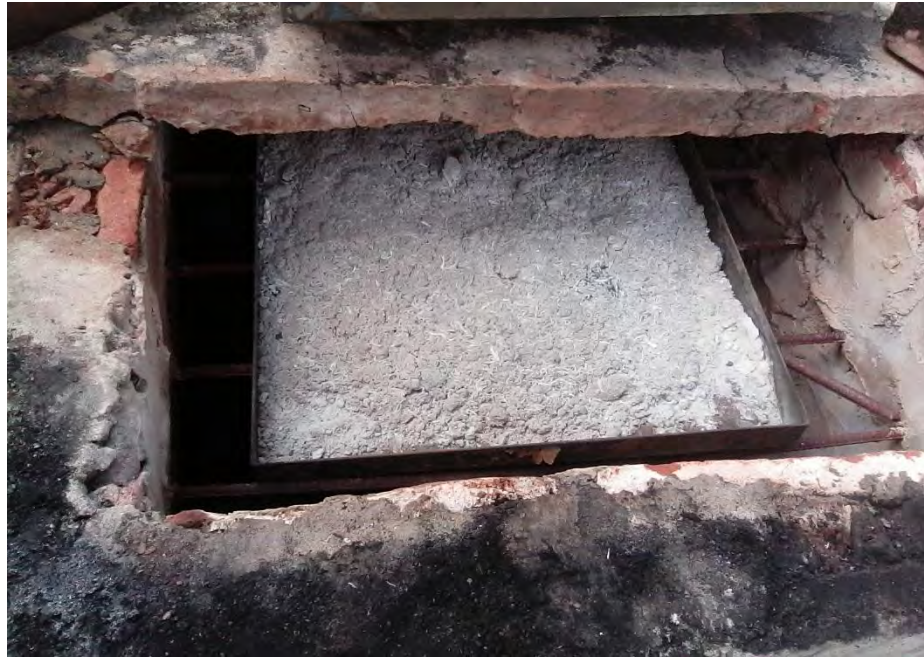
Figure A13 Local fresh bagasse ash after calcination in Brick furnace
