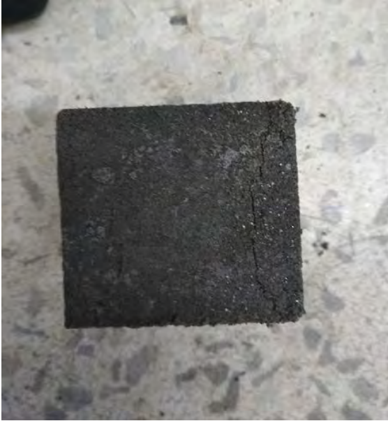
Figure A19 Bagasse ash blended cement mortar cube after failure
