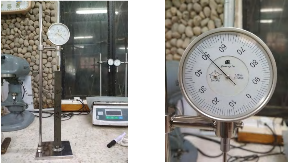
Figure 3.26: Comparator readings of test specimens
