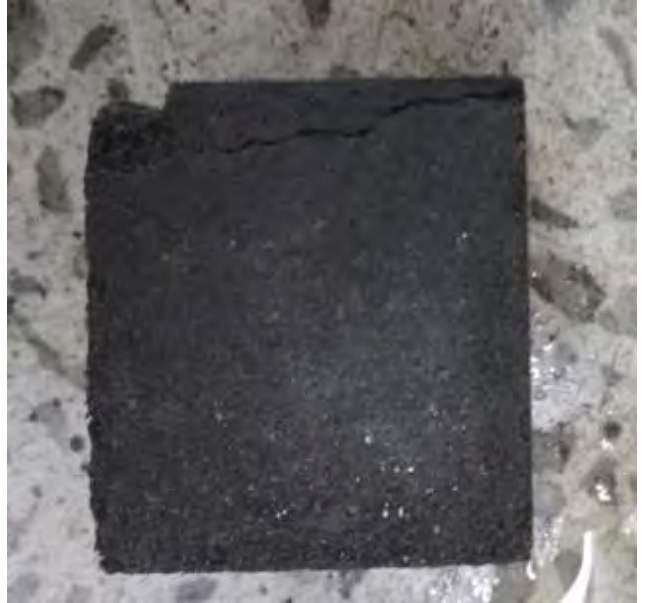
Figure A19 Bagasse ash blended cement mortar cube after failure
