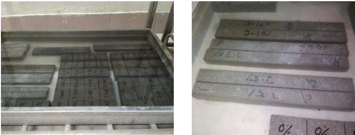
Figure 3.25: Curing of specimens for shrinkage test.
