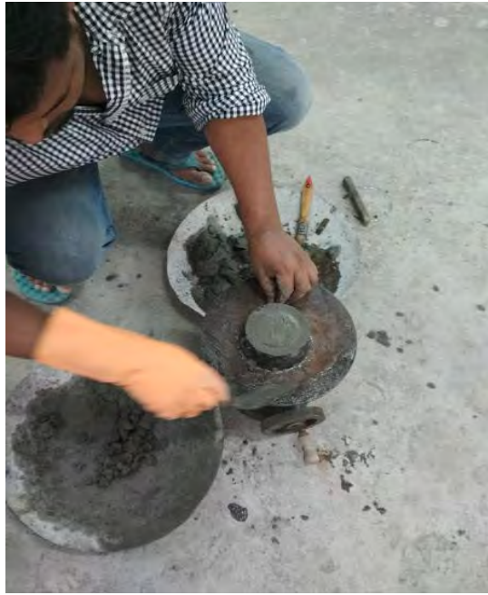
Figure A17 Placing of sample in the mold for flow test
