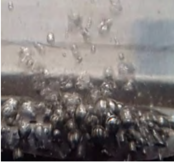
\Delta T = 20K; q = 92 \text{ kW/m}^2
