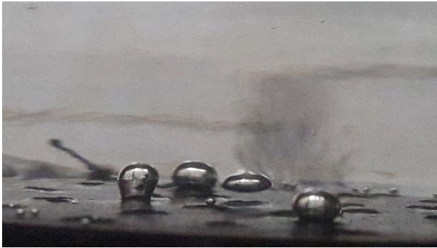
\Delta T = 2K; q = 5.50 \text{ kW/m}^2
