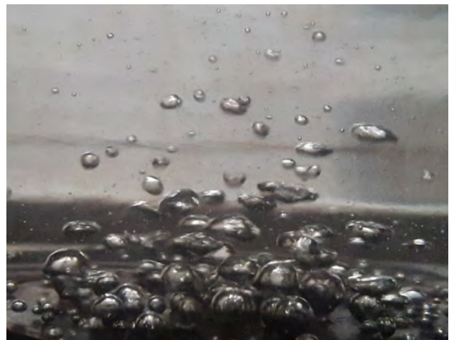
\Delta T = 28K ; q = 125 \text{ kW/m}^2
