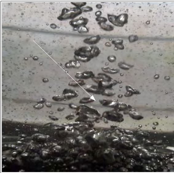
Fig. 4.9: Image obtained at 70 kW/m 2 on pitted surface showing the formation of buoyant column
