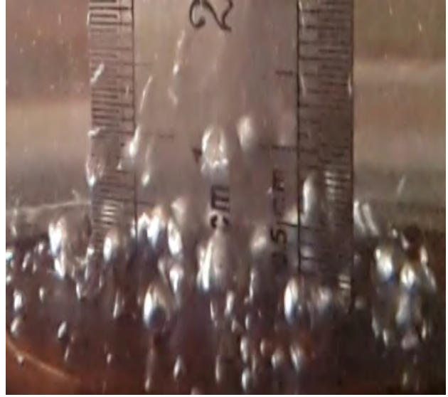
\Delta T = 14K; q = 50 \text{ kW/m}^2
