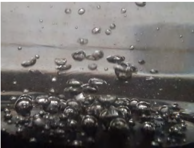
\Delta T = 16K; q = 102 \text{ kW/m}^2
