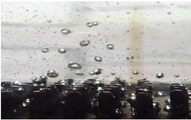
\Delta T = 2K; q = 17.6 \text{ kW/m}^2
