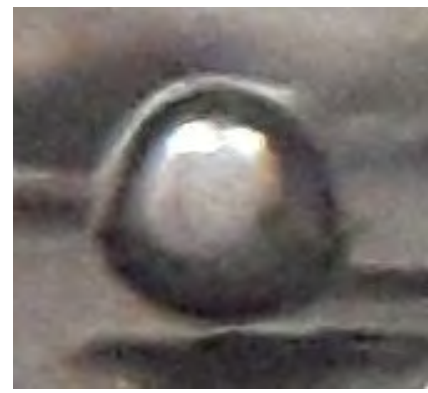
Detachment from the surface [t=130ms]
