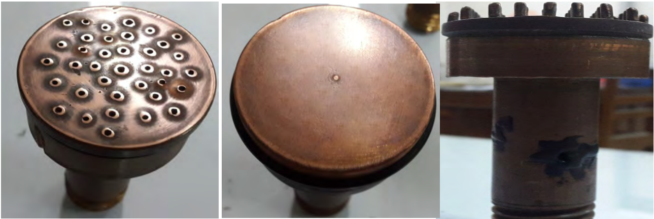
a) Pitted Surface
