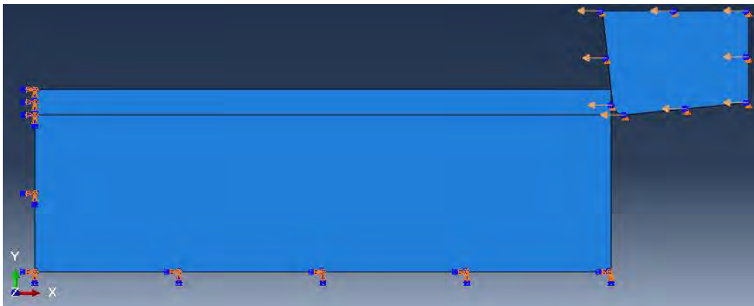
Fig.5.13 Boundary conditions of workpiece and tool
