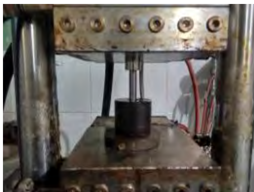
Figure 2.3.7. Pellets preparation method in hot press by compression molding
