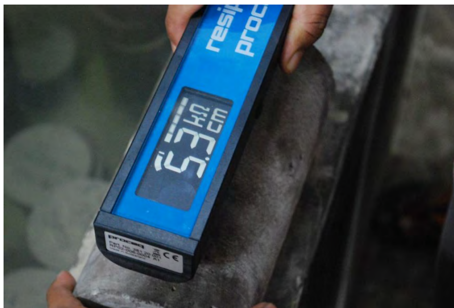
Figure 4.8: Concrete Resistivity Measurement using Proseq Resistod
