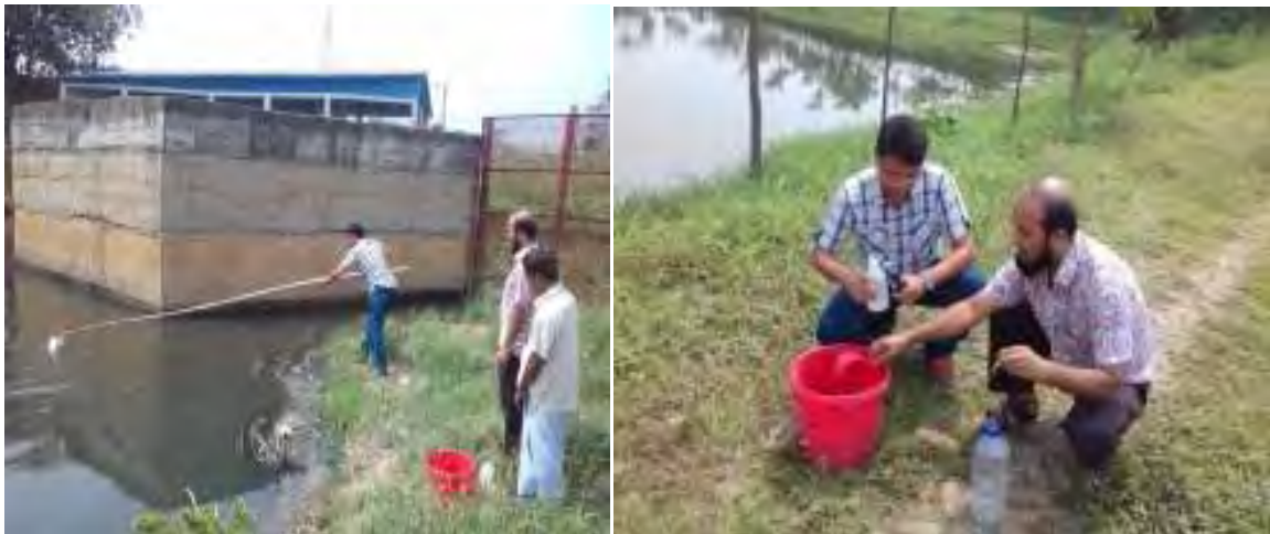
Fig 3.2 Collection of wastewater sample from the pit/manhole which receives sewer from both northern and southern sides of Hatirjheel.
