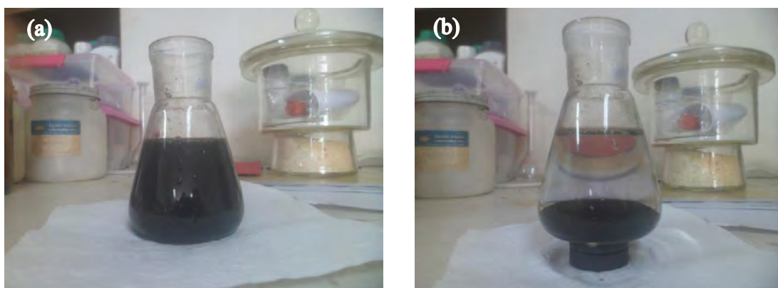
Fig. 4.11: Magnetic separation of \text{Fe}_3\text{O}_4 NPs (a) before applying magnetic field (b) after applying magnetic field
