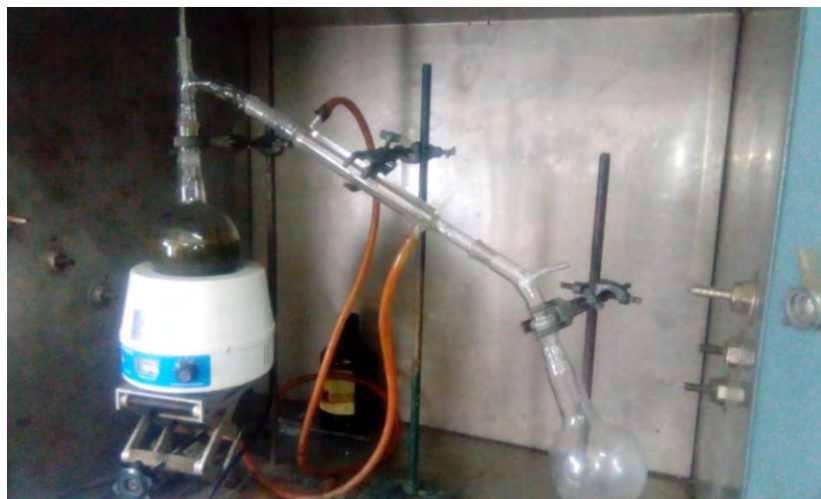
Fig. 4.7: Instrumental setup of essential oil collection from Ipomoea aquatica leaf extracts
