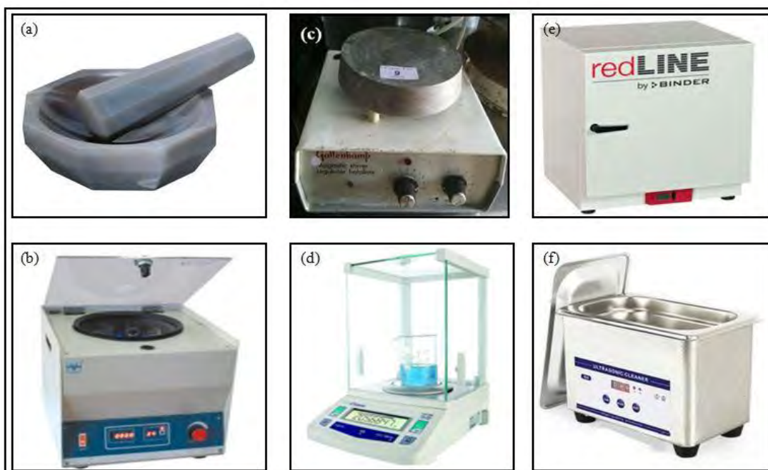
Fig. 4.1: Basic equipments used for synthesis of Fe 3 O 4 NPs (a) Mortar (b) Centrifuge machine (c) Magnetic stirrer (d) Digital balance (e) Electric oven (f) Bath sonicator
