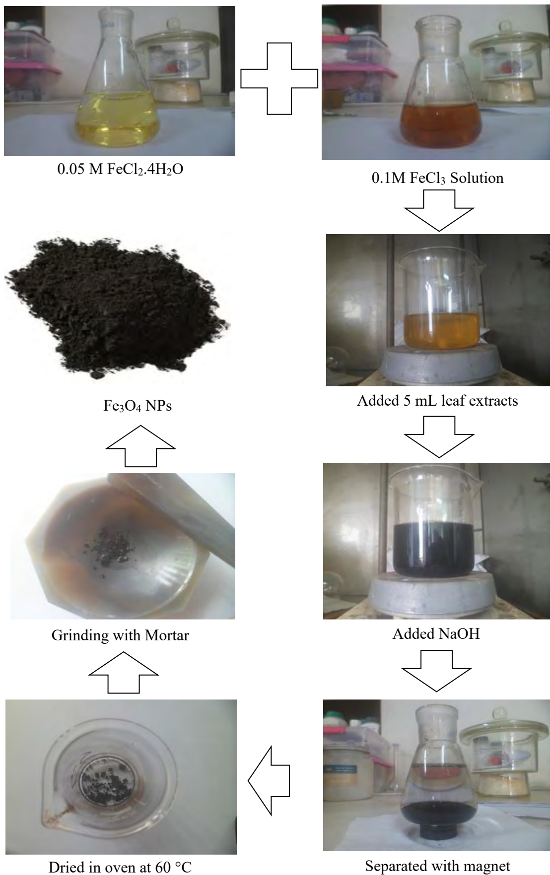
Fig. 4.12: \text{Fe}_3\text{O}_4 NPs synthesis
