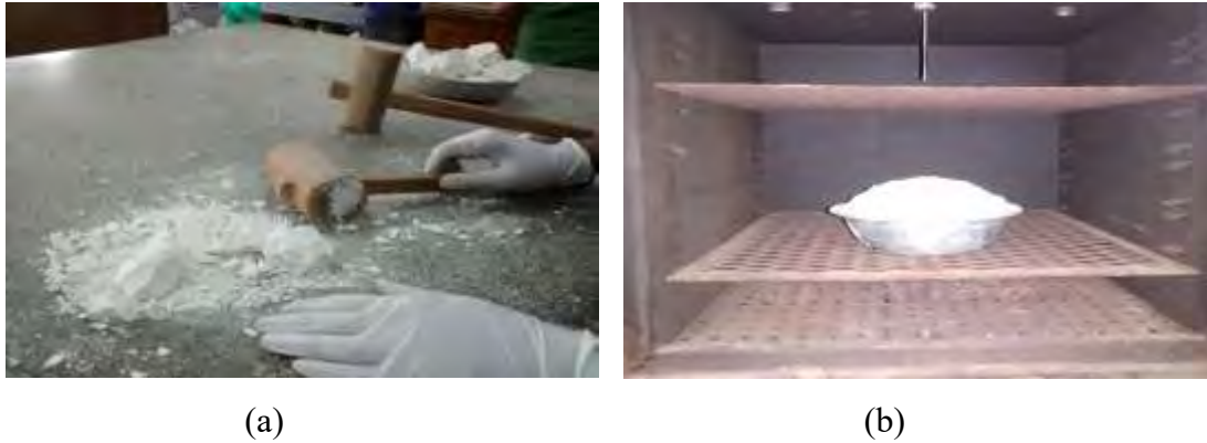
Figure 3.3: Photographs of preparing quicklime: (a) Grinding the limestone and (b) Oven drying of lime
