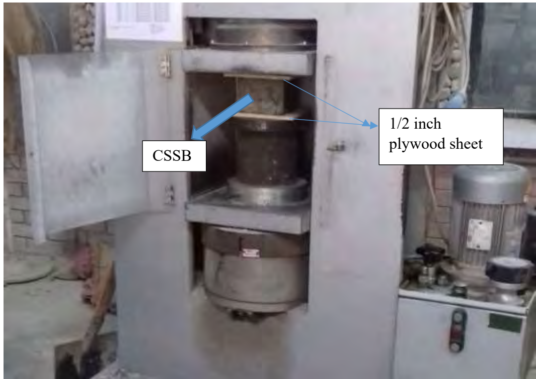
Figure 3.18: Photograph of CSSB specimen setup for crushing strength test
