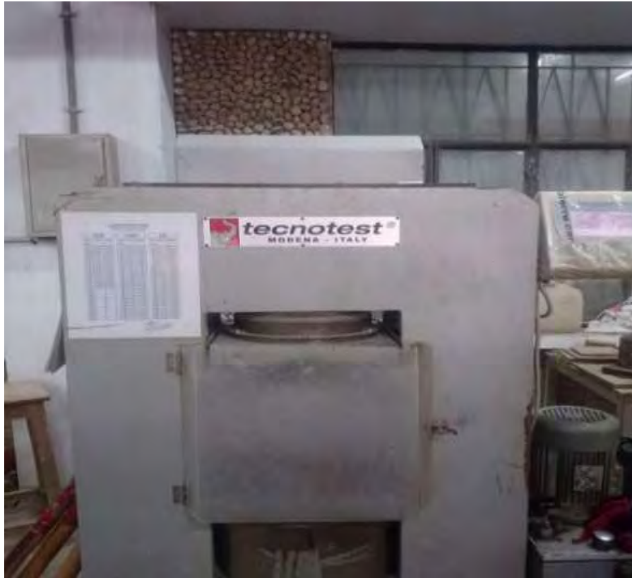
Figure 3.14: Photograph of crushing strength testing machine (Technotest Modena Italy)
