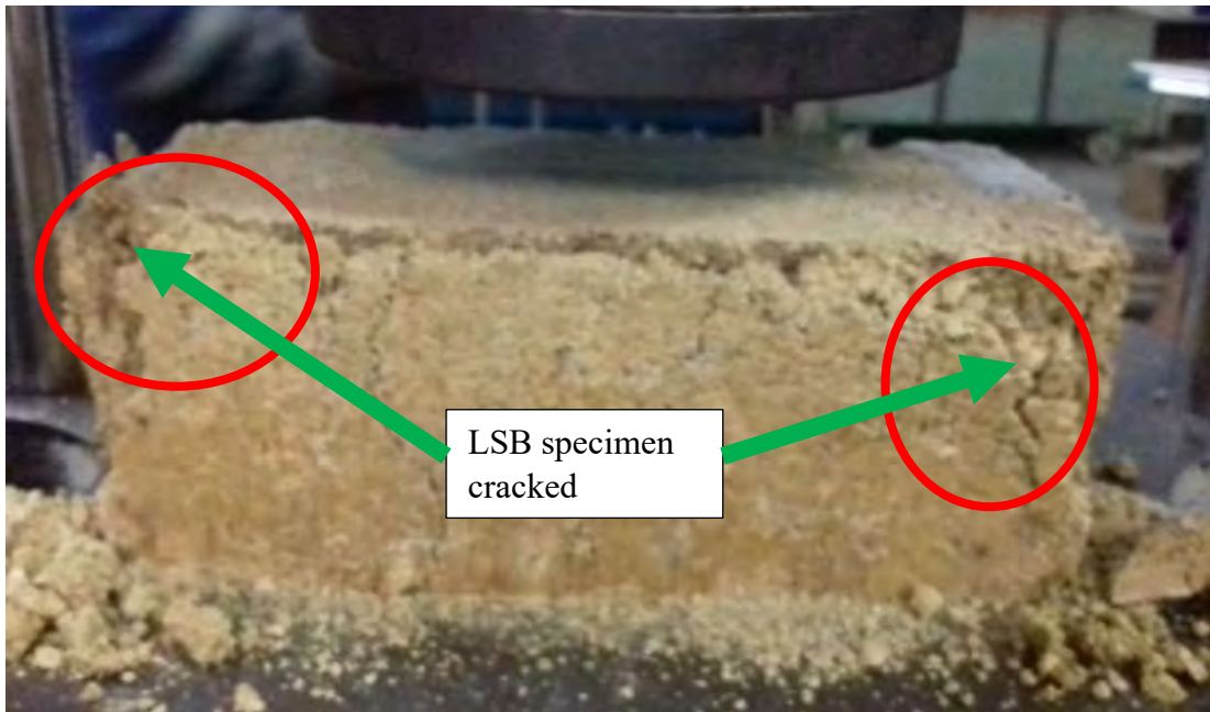
(c) Failure pattern of LSB specimen
