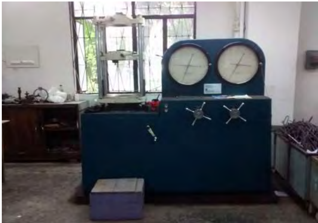
Figure 3.11: Photograph of Universal Testing Machine (Tinius Olsen Testing Machine Co. USA)
