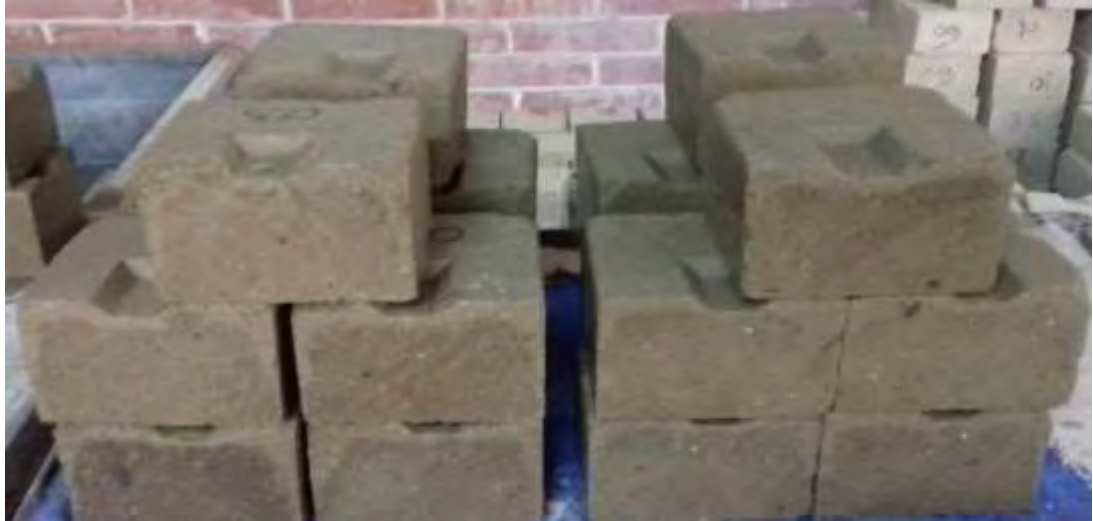
Figure 3.21: Photograph of wet CSSB specimens after 24 hours immersion under water
