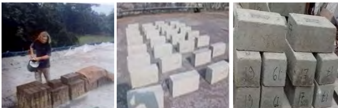
(g) Curing by water (h) Curing in open air (i) Block after curing
