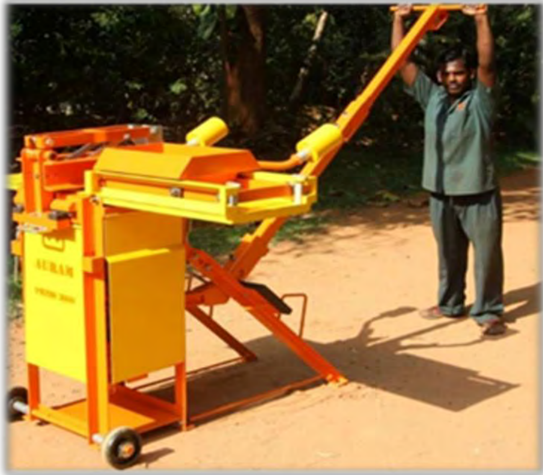
Figure 3.8: Block producing machine: “Auram Earth Block Press 3000”
