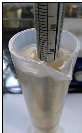
Fig. 3.8 Density was tested by deeping the hydrometer in the liquid.
