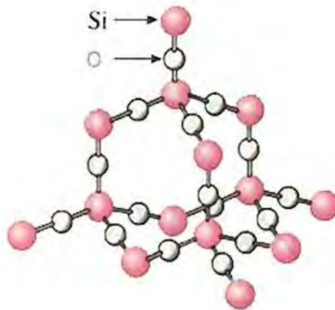
Fig. 2.4 Structure of precipitated silica [20].
