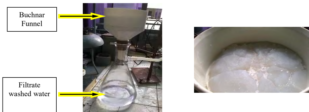
Fig. 3.11 (a) Separation of silica by filtration; (b) Wet precipitated silica after filtration.
