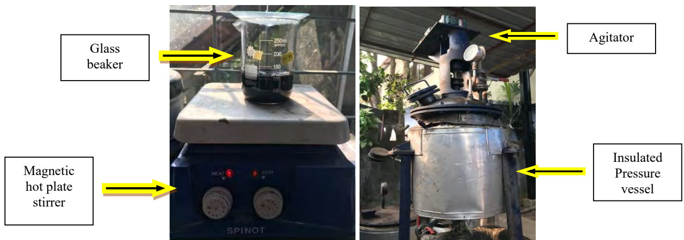
Fig. 3.5 Alkali extraction in laboratory glass beaker and in pilot digester.
