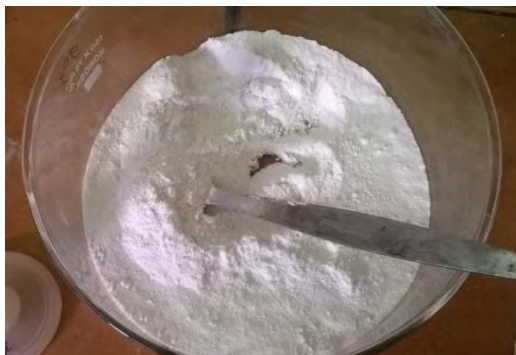
Fig. 3.13 Precipitated silica powder after drying and milling.
