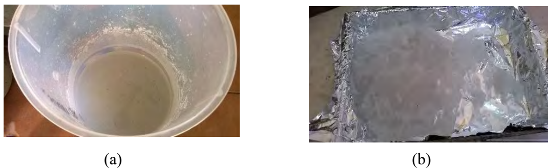
Fig. 3.12 (a) Formation of transparent gel solution; (b) Transparent solid gel after filtration.
