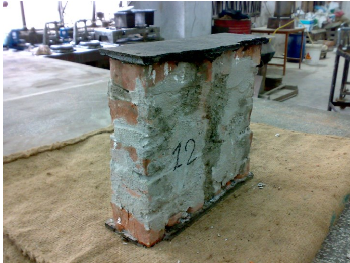
Figure D.12(a) Specimen-12: Maximum Load= 10.10 Ton
