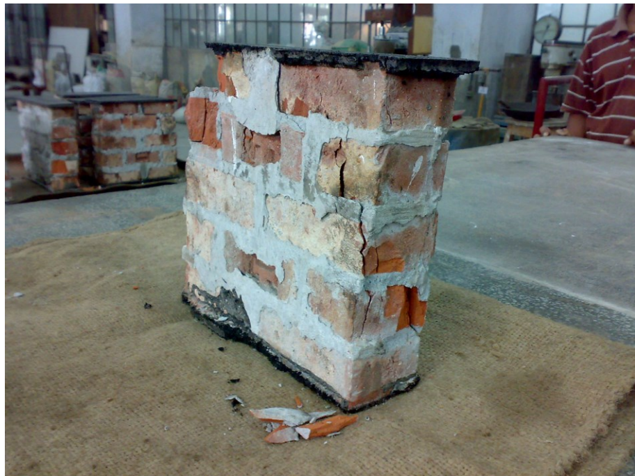
Figure D.7(b) Specimen-7: Maximum Load=14.26Ton
