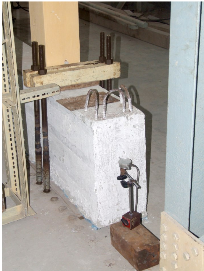
Figure 3.11 Location of displacement transducer to measure the base movement of the specimens
