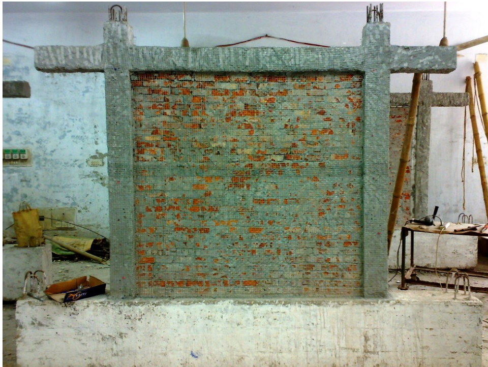
Figure 3.28(a) Wiremesh wrapped around the RC frame and the infill
