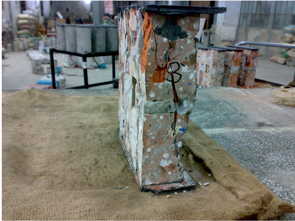
Figure D.3(a) Specimen-3: Maximum Load=12.18 Ton
