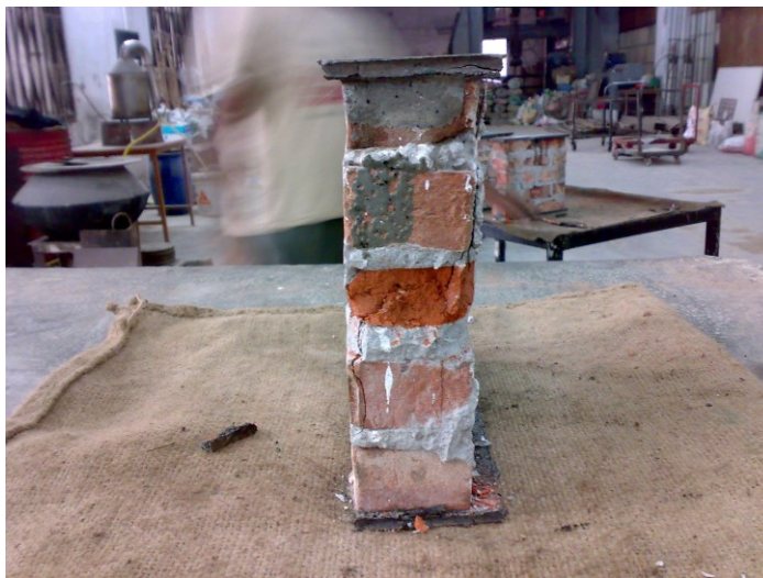
Figure D.10(b) Specimen-10: Maximum Load= 17.41 Ton
