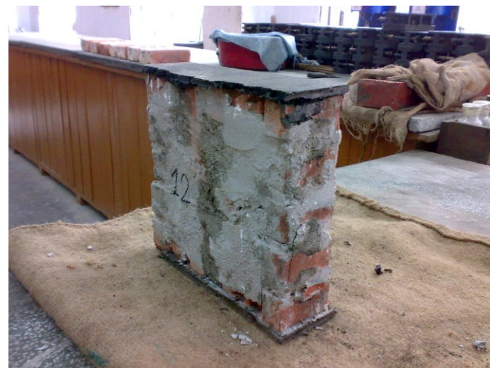
Figure D.12(c) Specimen-12: Maximum Load= 10.10 Ton
