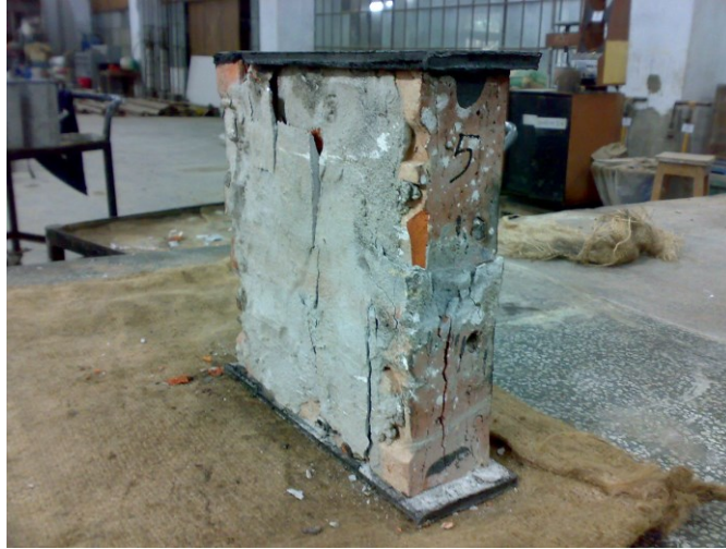
Figure D.5(a) Specimen-5: Maximum Load=12.18 Ton
