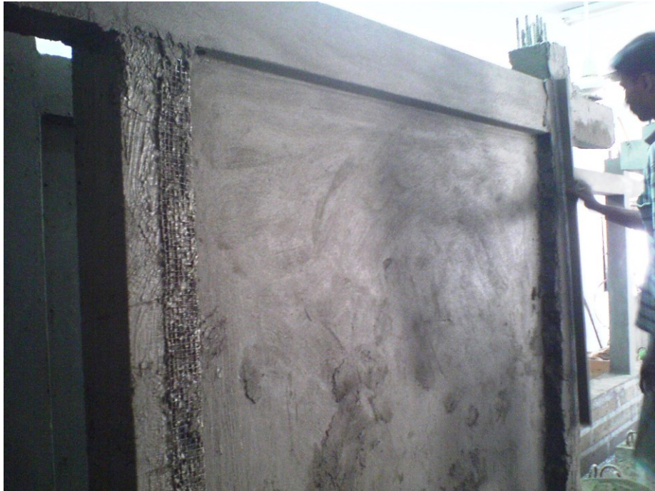
Figure 3.22 Surface finishing of the isolated brick infilled RC frame specimen
