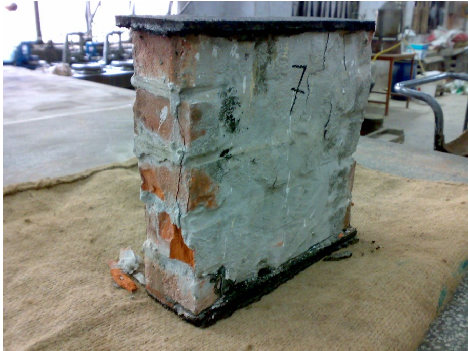
Figure D.7(a) Specimen-7: Maximum Load=14.26Ton
