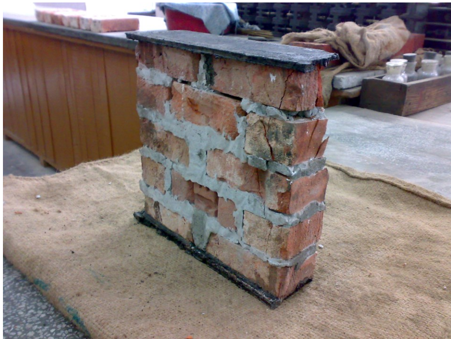
Figure D.8(b) Specimen-8: Maximum Load=10.10 Ton
