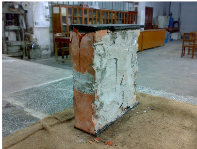
Figure D.5(c) Specimen-5: Maximum Load=12.18 Ton
