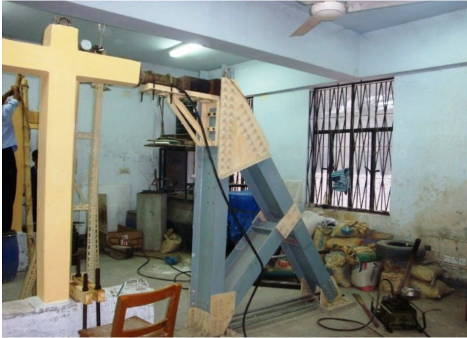
Figure 3.5 Reaction frame and the position of hydraulic jack
