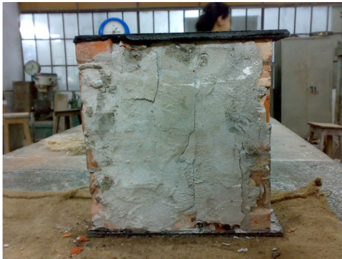
Figure D.5(b) Specimen-5: Maximum Load=12.18 Ton
