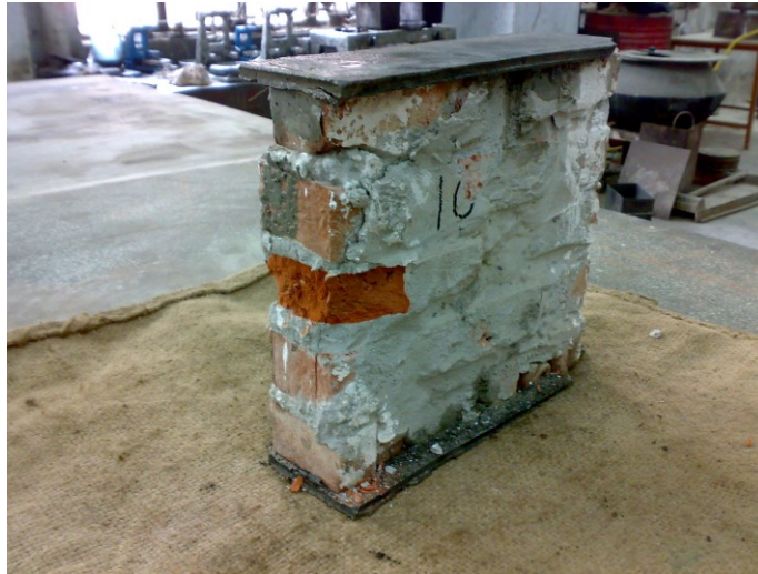
Figure D.10(a) Specimen-10: Maximum Load= 17.41 Ton
