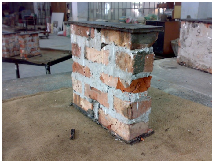
Figure D.10(c) Specimen-10: Maximum Load= 17.41 Ton
