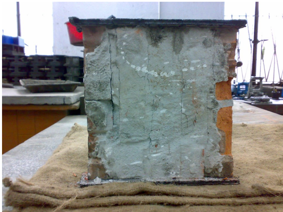
Figure D.3(b) Specimen-3: Maximum Load=12.18 Ton
