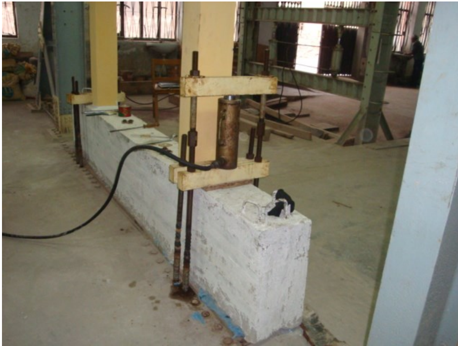
Figure 3.3 Pre-tensioning of anchor bolts using hydraulic jack to ensure the fixity of the specimen along the strong base
