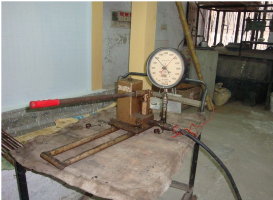
Figure 3.6 Dial gauge and pumper attached with the hydraulic jack
