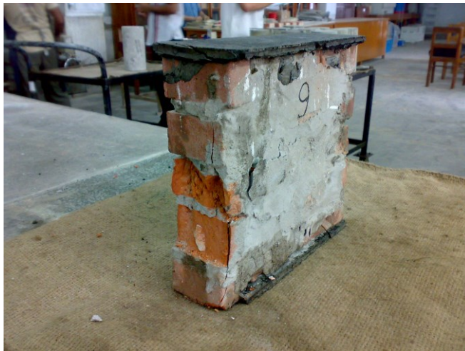
Figure D.9(b) Specimen-9: Maximum Load= 8.02 Ton
