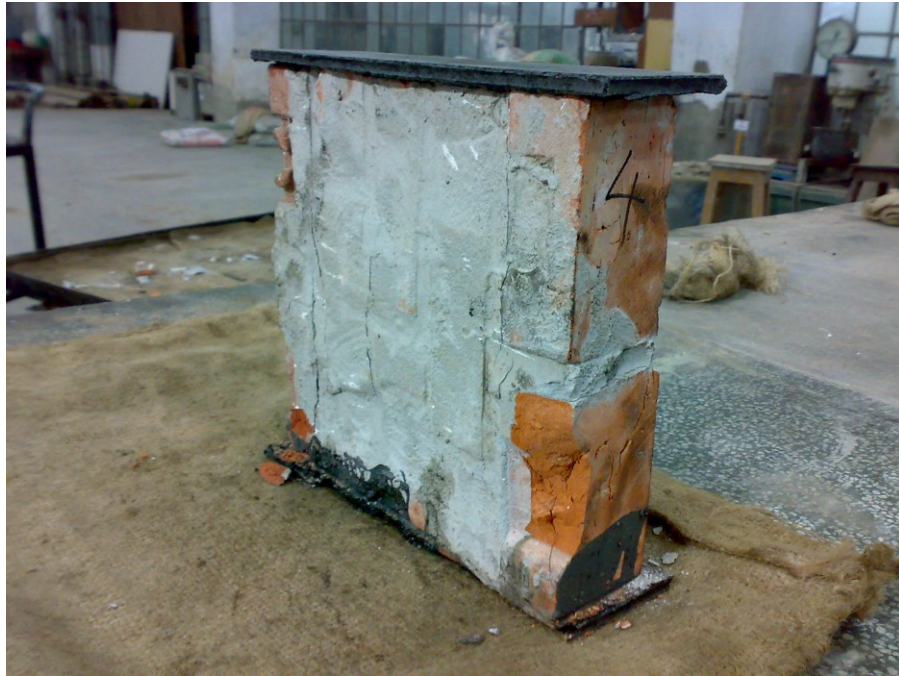
Figure D.4(a) Specimen-4: Maximum Load=17.39Ton
