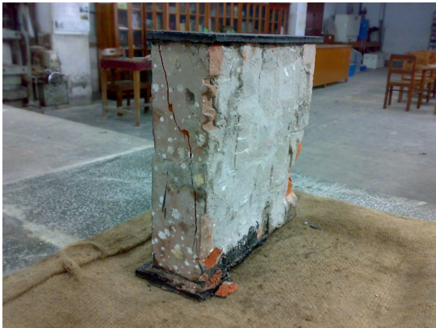
Figure D.4(b) Specimen-4: Maximum Load=17.39Ton
