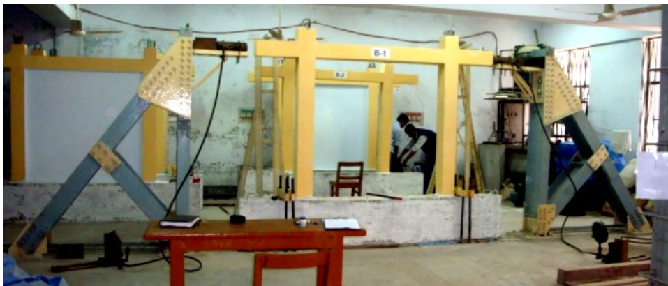
(b) In-plane cyclic load test of bare RC frame
