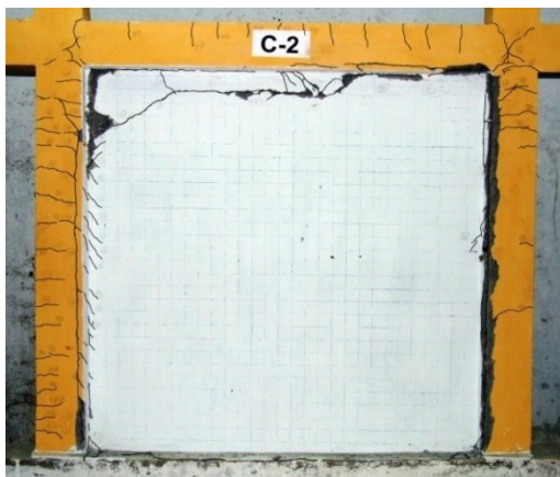
(c) Repaired isolated brick infilled RC frame
