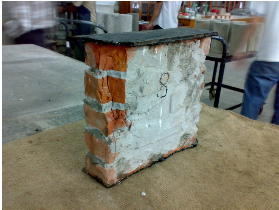
Figure D.8(a) Specimen-8: Maximum Load=10.10 Ton
