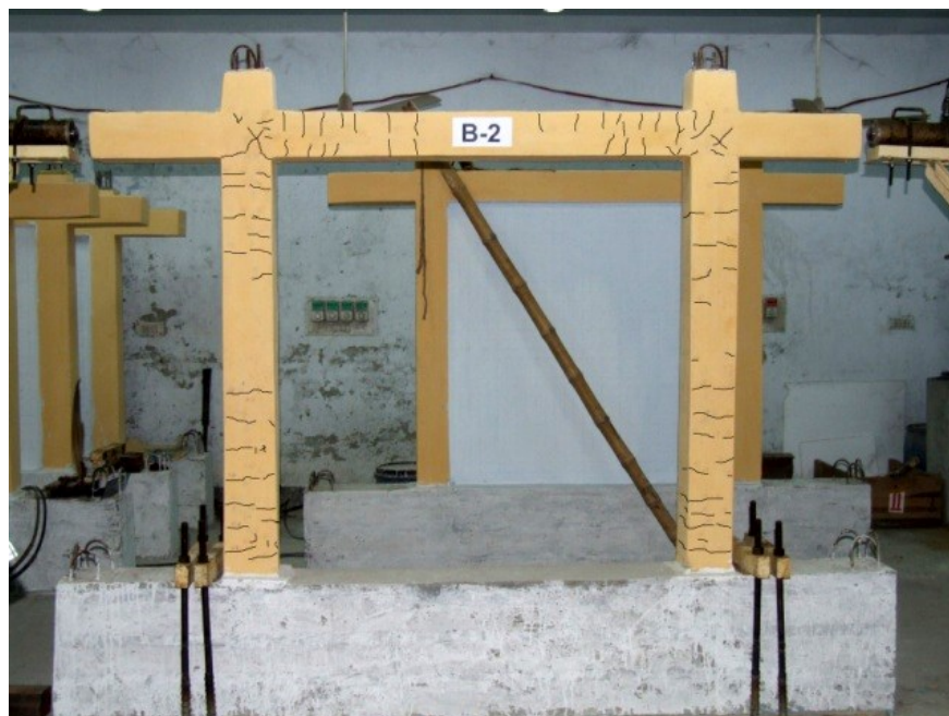
Figure 4.7(b) Crack patterns at maximum lateral load in RC Bare frame in specimen B2
