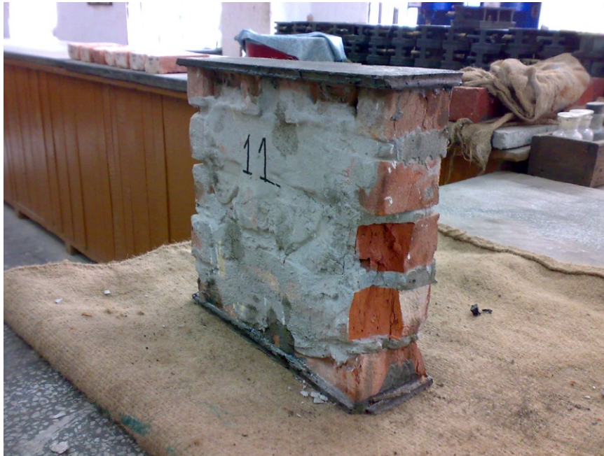
Figure D.11(a) Specimen-11: Maximum Load= 18.95 Ton
