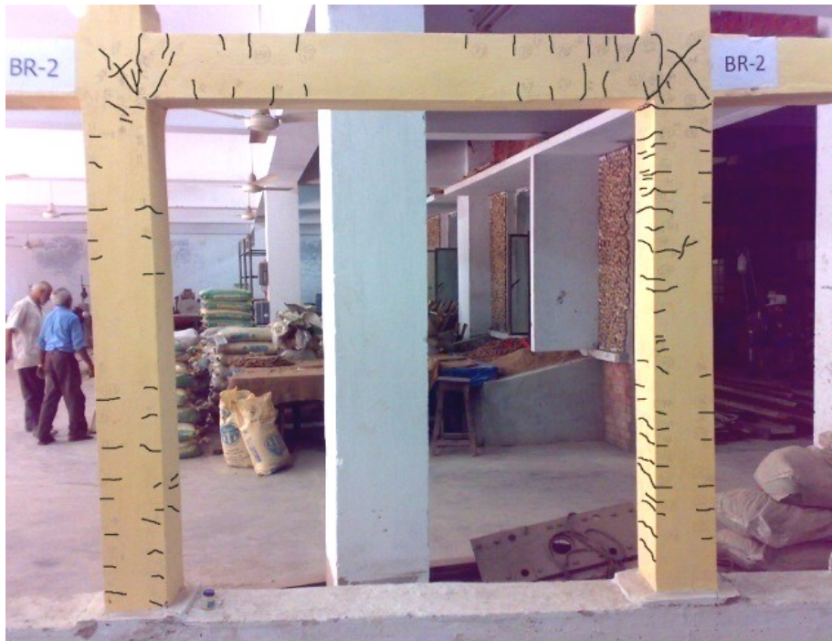
Figure 4.8(b) Crack patterns at peak load in repaired RC Bare frame specimen BR2
