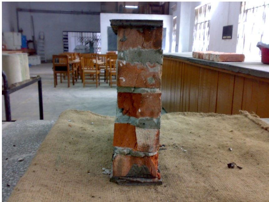
Figure D.11(b) Specimen-11: Maximum Load= 18.95 Ton
