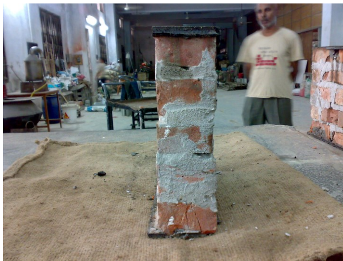
Figure D.12(b) Specimen-12: Maximum Load= 10.10 Ton
