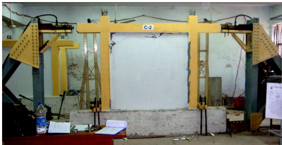
(c) In-plane cyclic load test of isolated infilled RC frame
