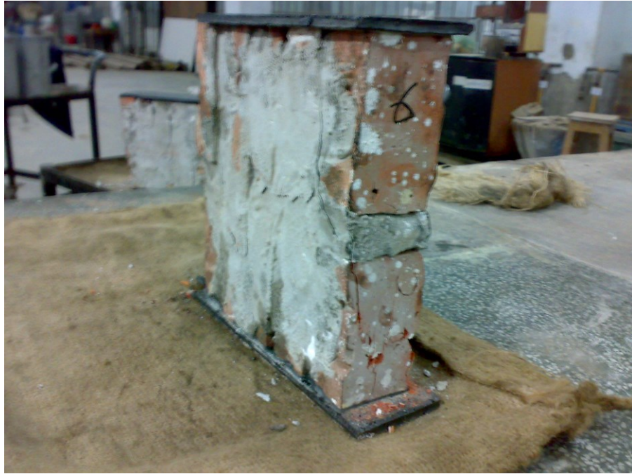
Figure D.6(a) Specimen-6: Maximum Load=20.51Ton
