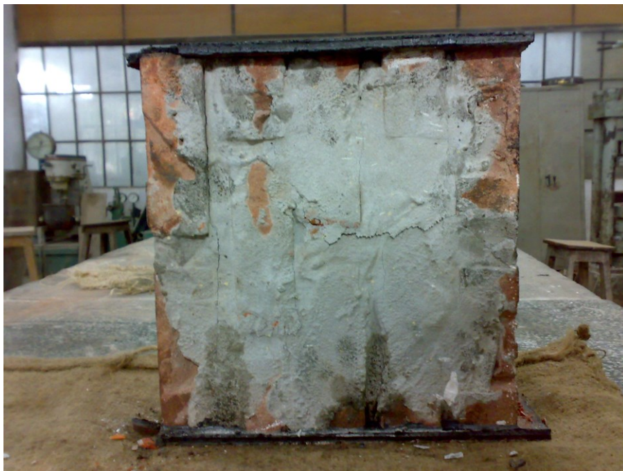
Figure D.6(b) Specimen-6: Maximum Load=20.51Ton
