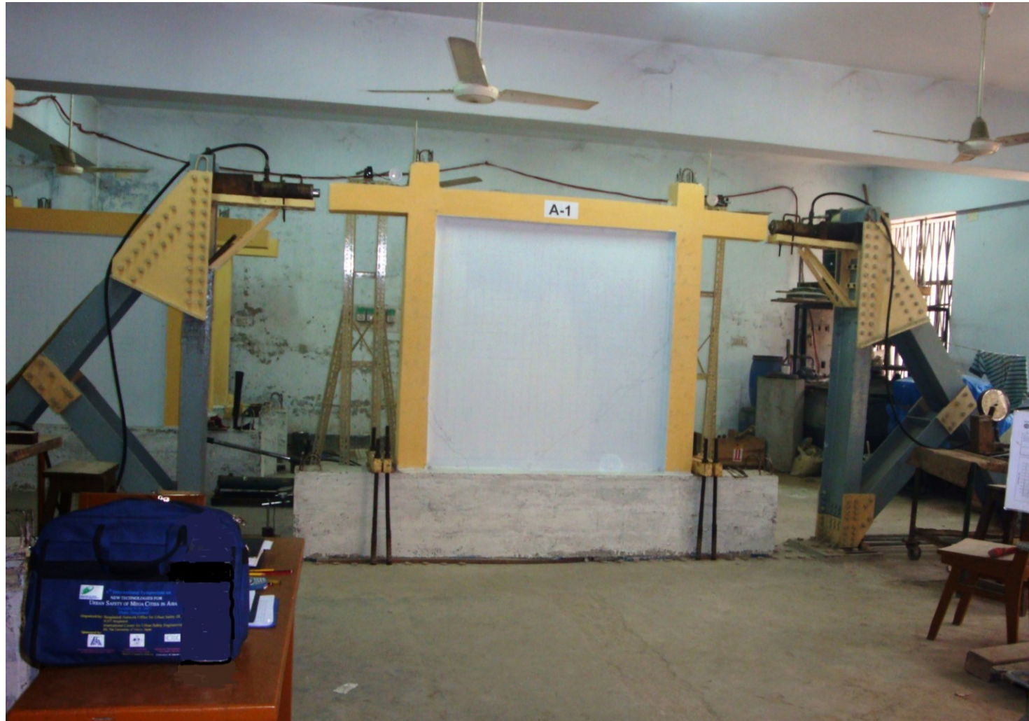
Figure 3.2 In-plane cyclic loading test setup in BUET, Bangladesh
