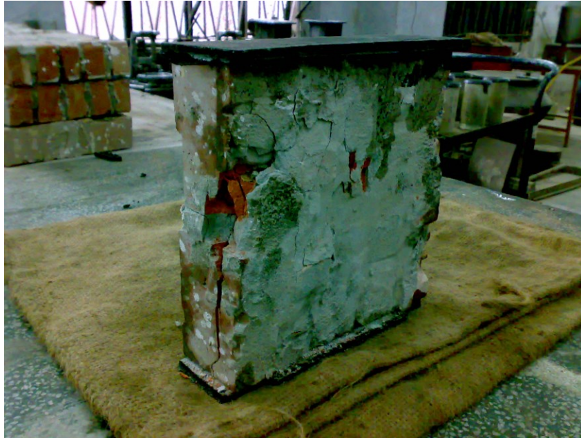
Figure D.1 Specimen-1: Maximum Load=19.74 Ton
