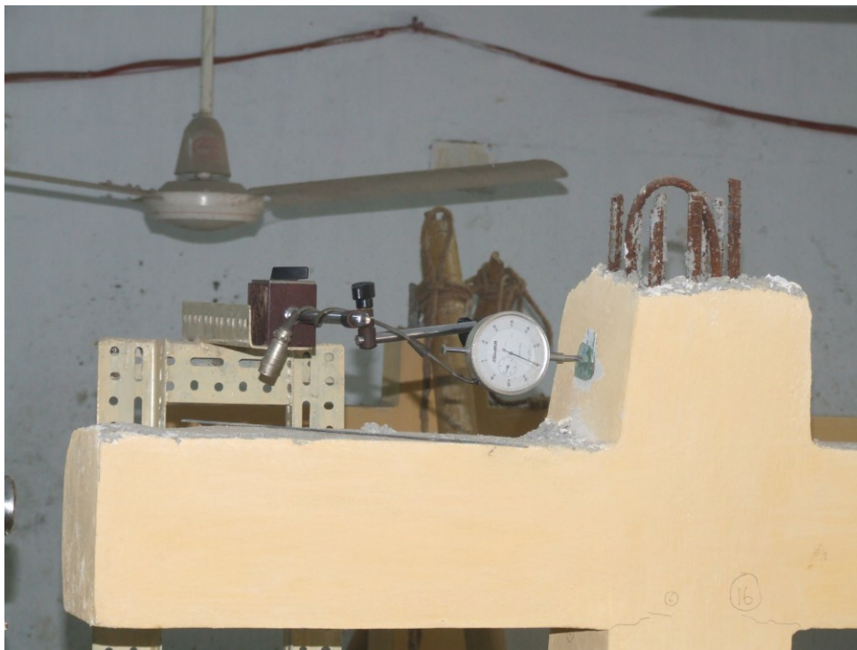
Figure 3.9 Mounting of displacement transducers to measure the top deflections
