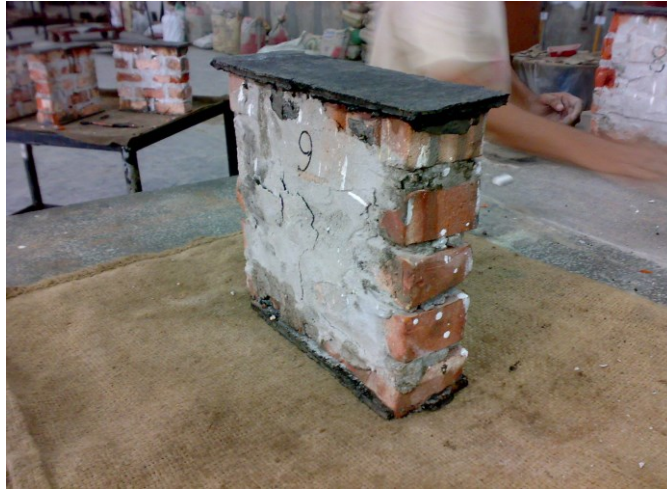
Figure D.9(a) Specimen-9: Maximum Load= 8.02 Ton
