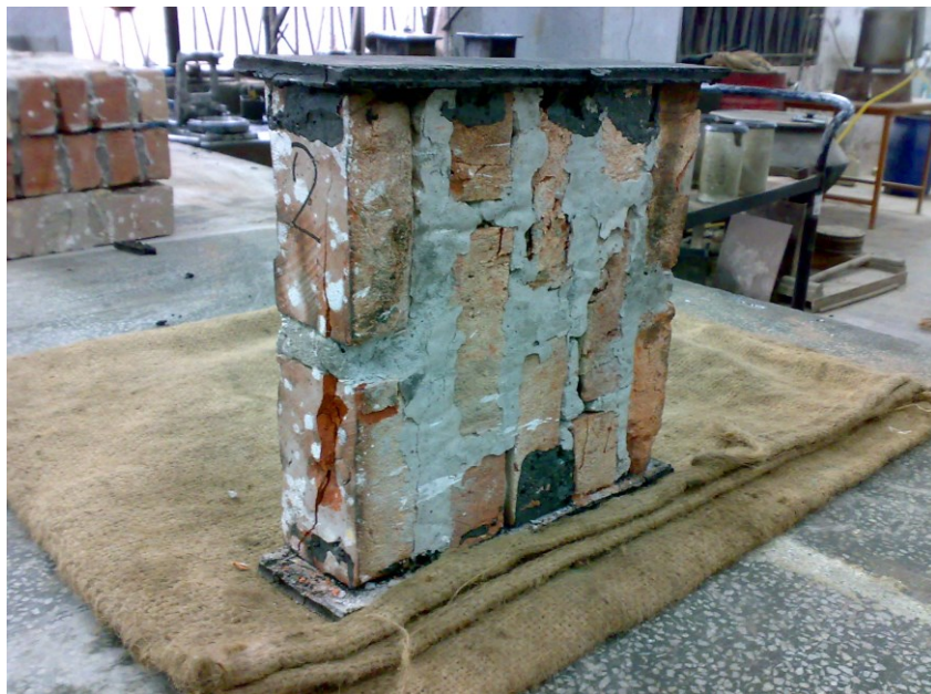
Figure D.2 Specimen-2: Maximum Load=21.55 Ton
