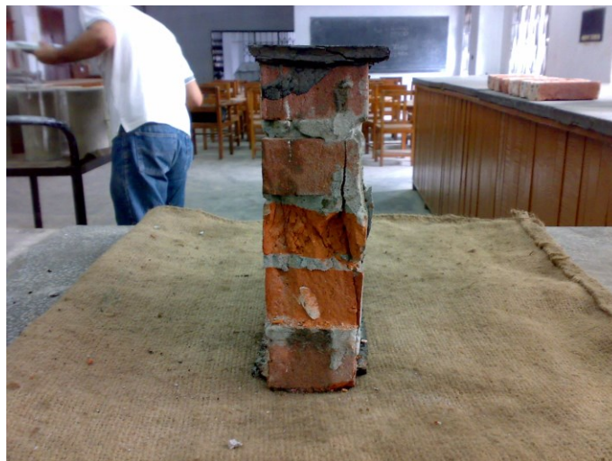
Figure D.9(c) Specimen-9: Maximum Load= 8.02 Ton
