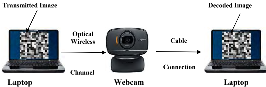
Fig. 6.1: Schematic diagram of practical pixelated communication system
