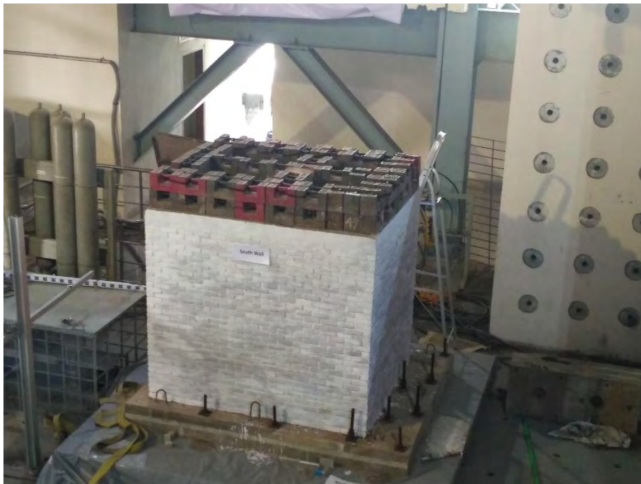
Figure 3.9 Weights on the slab
