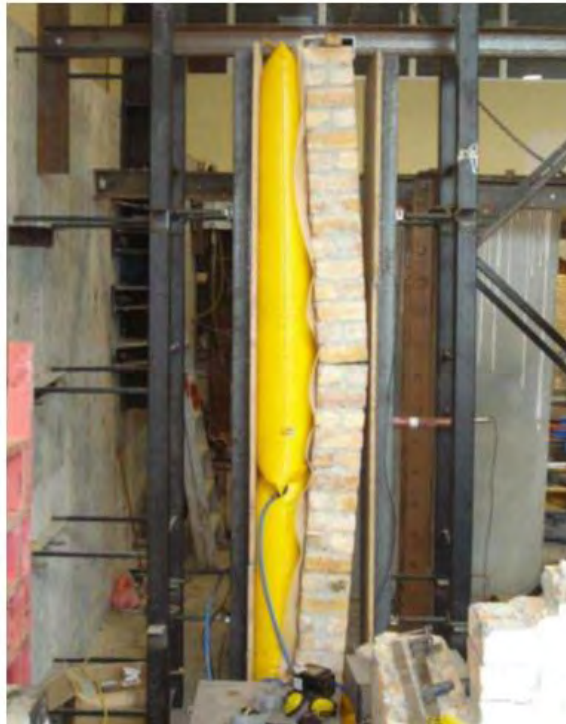
Figure 2.14 Test Setup for out of plane test of masonry wall (Derakhshan and Ingham, 2008)
