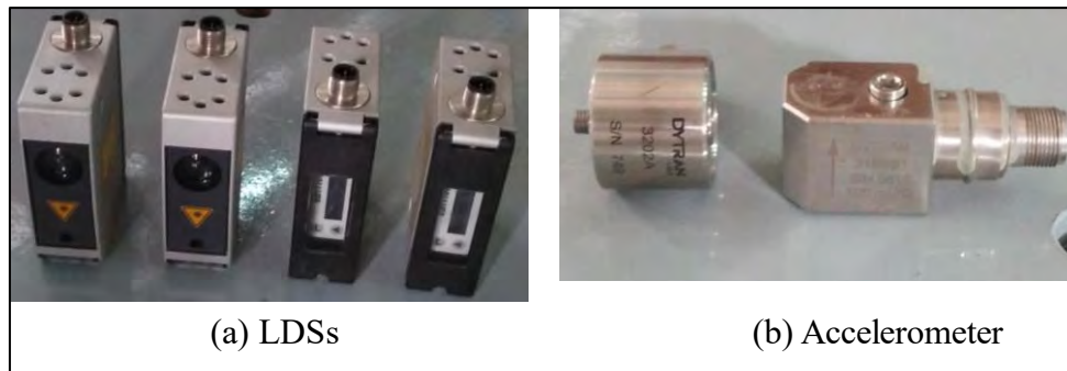
Figure 3.11 Instruments used in the test
