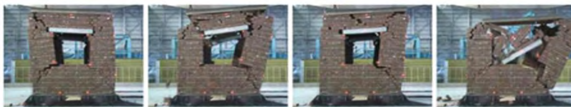
Figure 2.11 Process of specimen collapse in the shaking table test (Nakagawa et.al., 2012)
