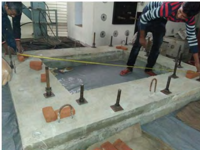
Figure 3.5 Foundation pad on shake table
