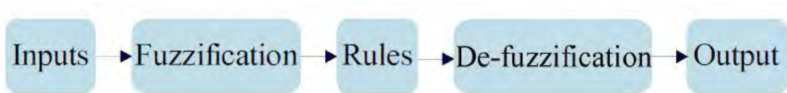
Fig. 2.8: Flowchart algorithm for MPPT method based on Fuzzy logic.
