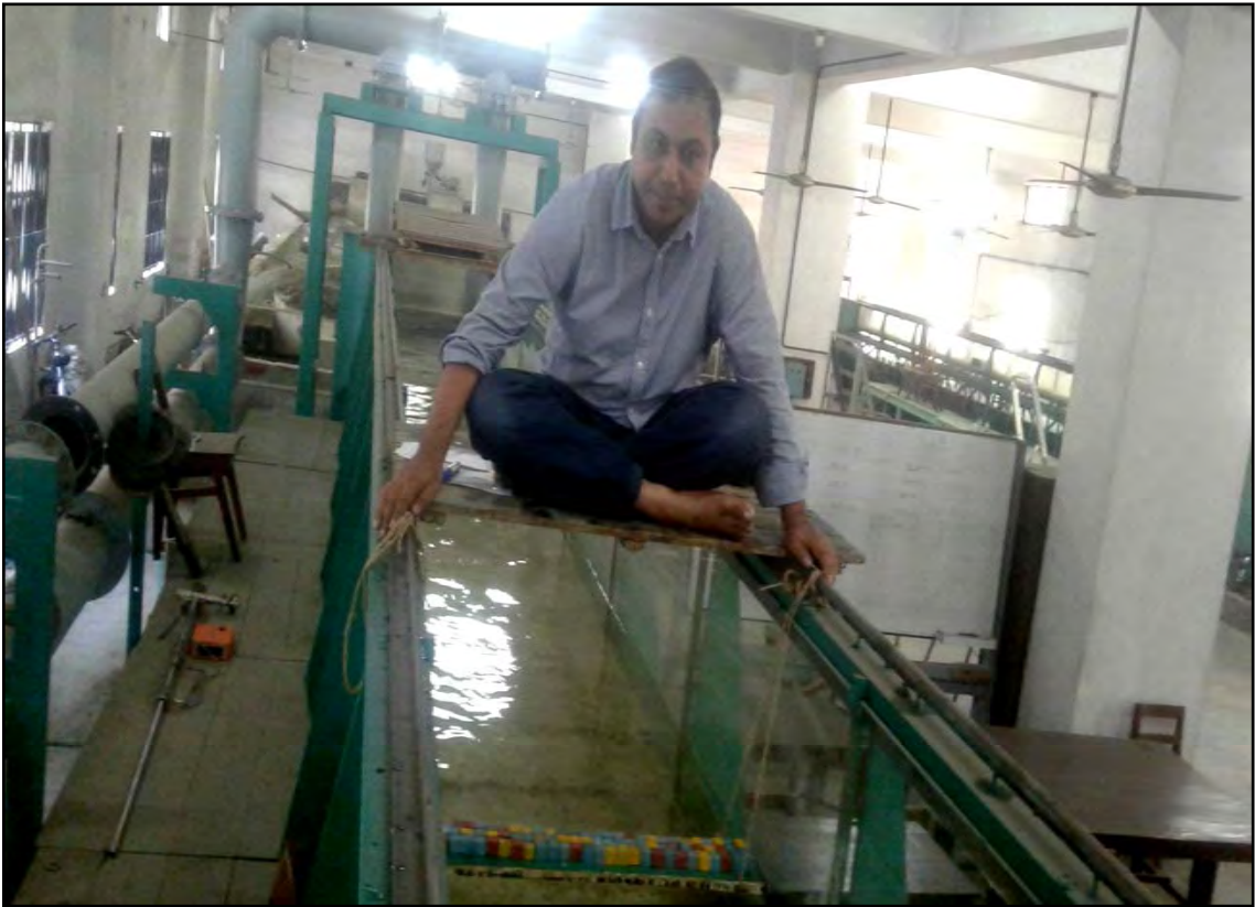
Photograph 3.9: Dumping of CC block to construct apron in the flume.
