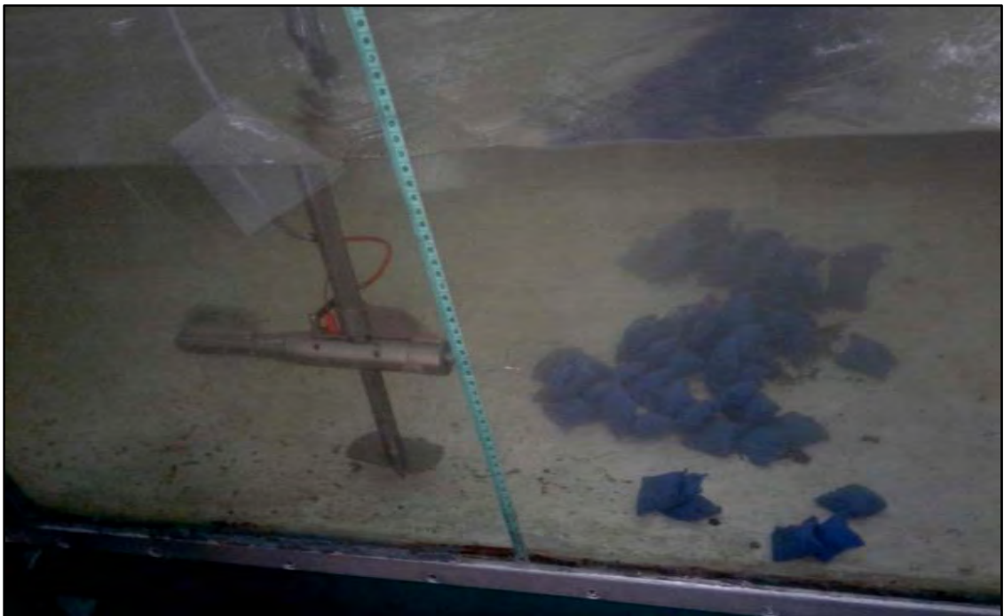
Photograph 3.8: Measurement of incipient velocity for geobags.
