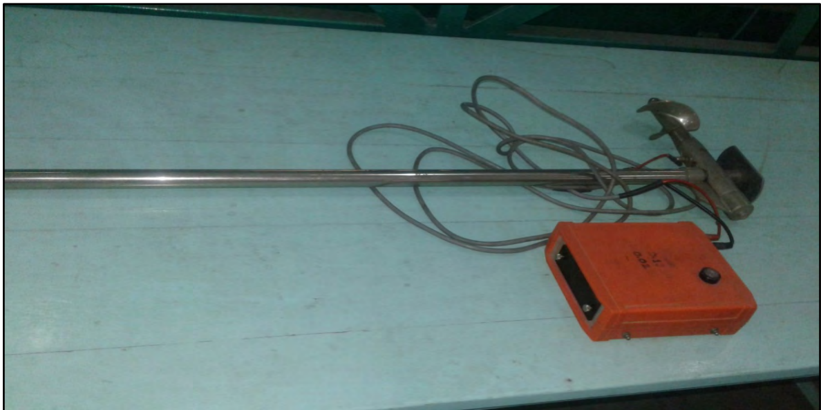
Photograph 3.3: Velocity measurement using current meter.
