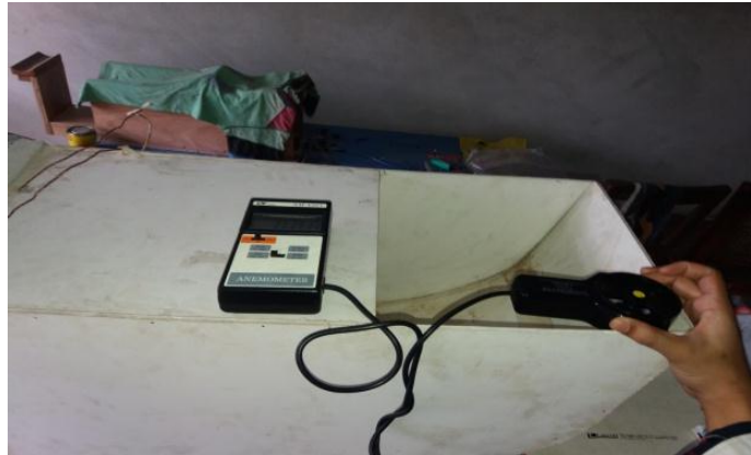
Figure 40: Measurement of air flow rate at different positions
