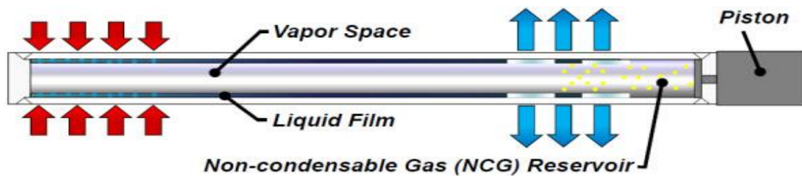
Figure 6: Pressure controlled heat pipe (PCHP) [17]
