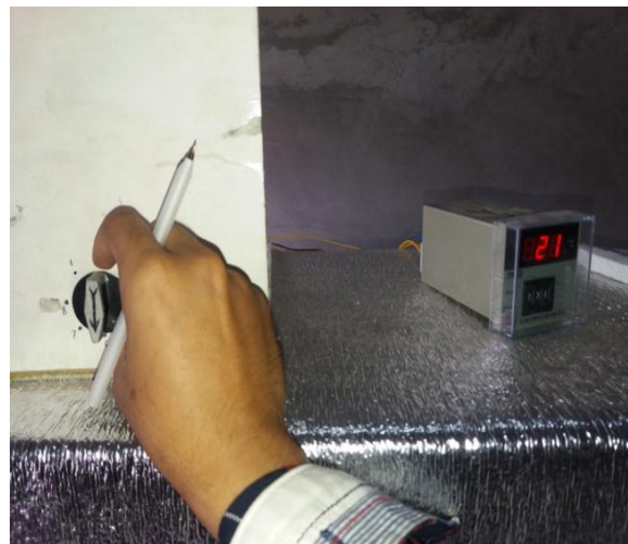
Figure 41: Measurement of temperature by thermocouple and selector switch
