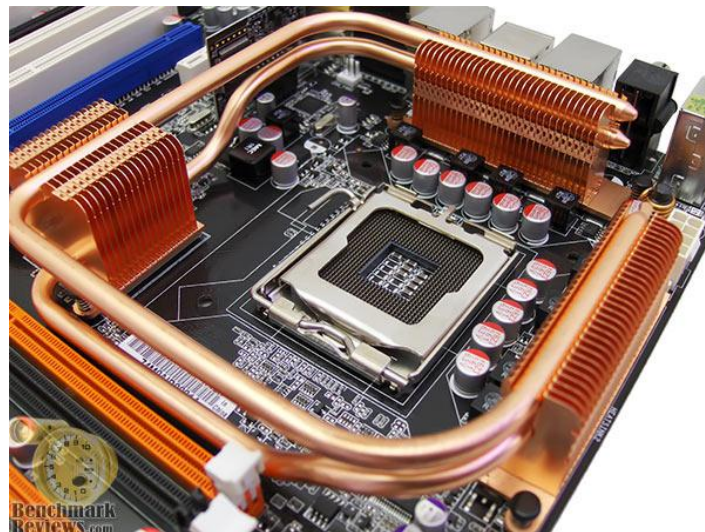
Figure 11: Heat pipe cooling device [45]
