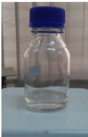
Fig. 3.1 Clear, viscous 17 wt% CA solution in 3:1 acetic acid/water stirred for 4 hrs
