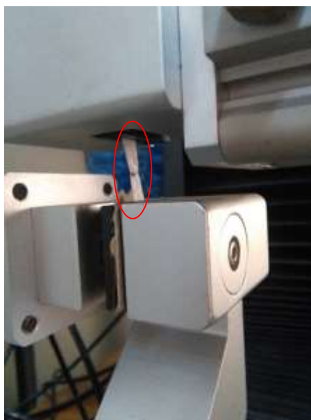
Fig. 6.6 Failure of the CA fibre mat during tensile test
