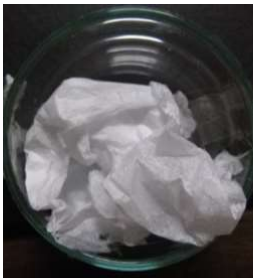
Fig. 3.3 Collected CA fibre mat after electrospinning
