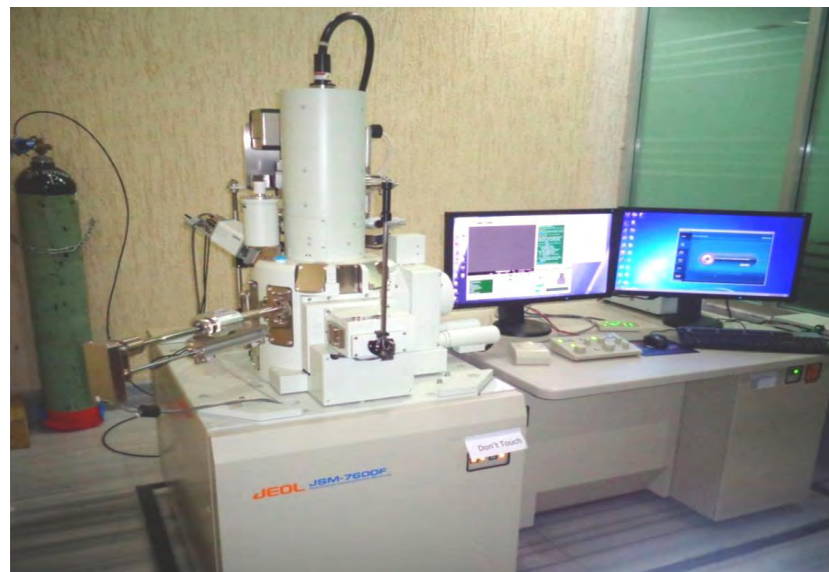
Figure 3.3: A field emission scanning electron microscope set up
