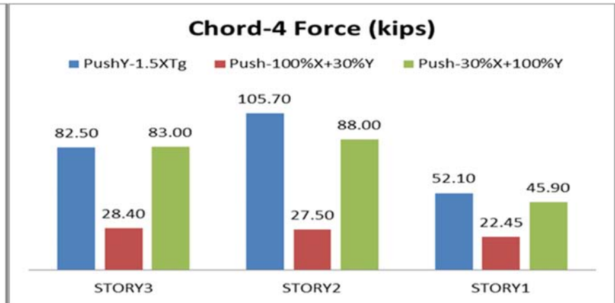
Figure 5-40 Chord-4 force (kips) of Model-2 from Pushover Analyses
