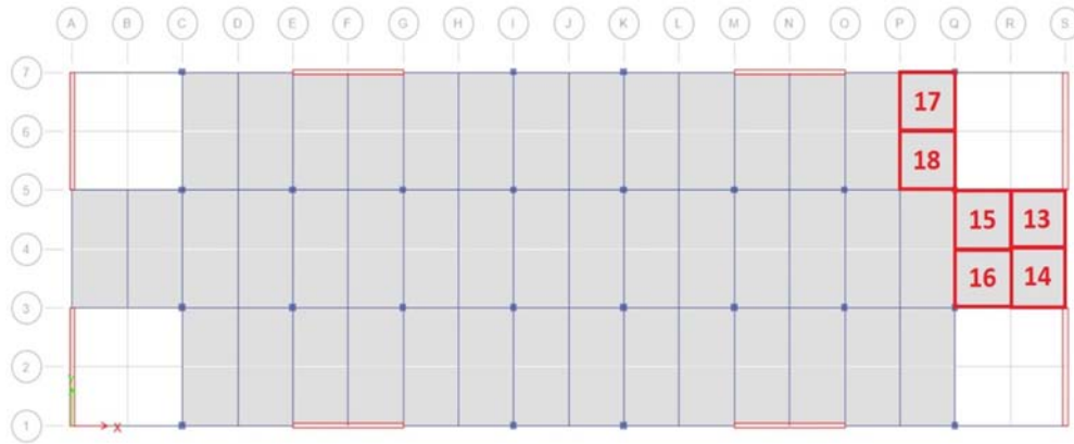
Figure 4-9 Diaphragm locations under consideration for investigation of shell layer stress of Model-5
