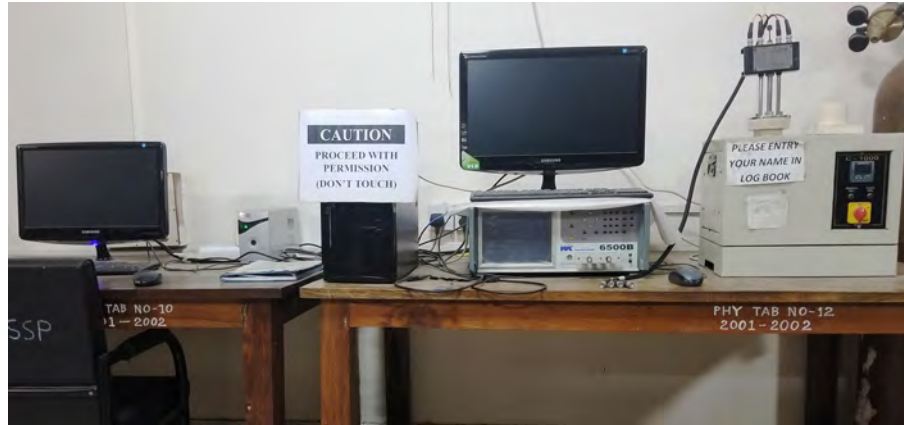
Fig. 4.11: Experimental setup of Wayne Kerr Impedance Analyzer (6500B).
