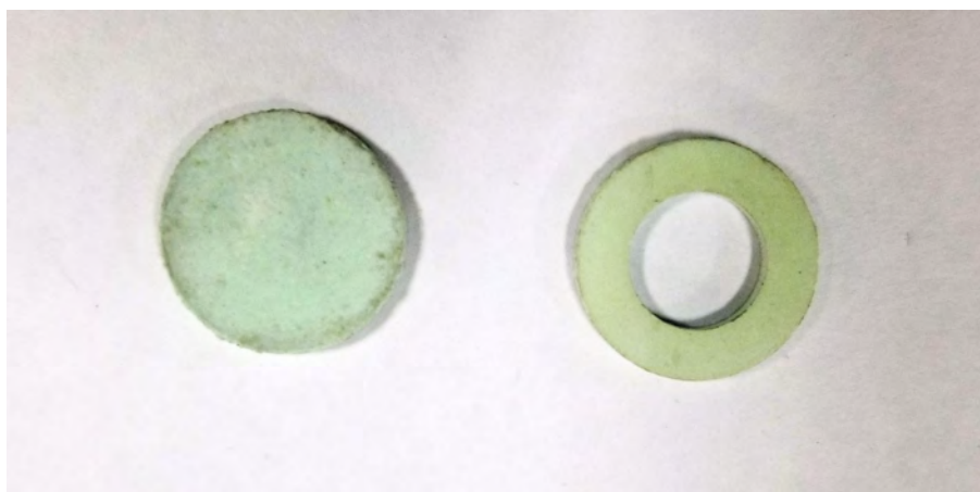
Fig. 3.7: Cylindrical and toroid shaped green body.
