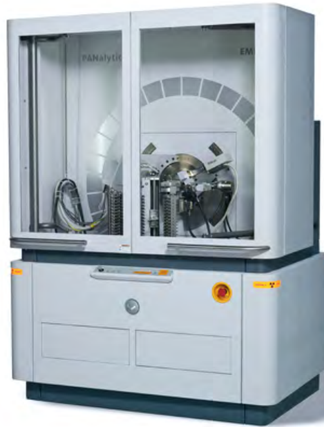
Fig. 4.3: A typical X-ray diffractometer used for XRD [5].
