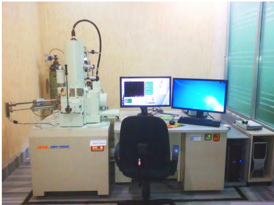
Fig. 4.6: Field emission scanning electron microscope (FESEM) setup.
