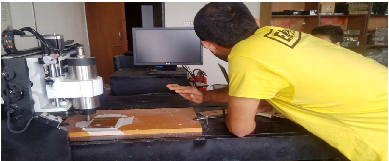
Figure 4.13: Drilling monitoring of PCB by CNC machine.
