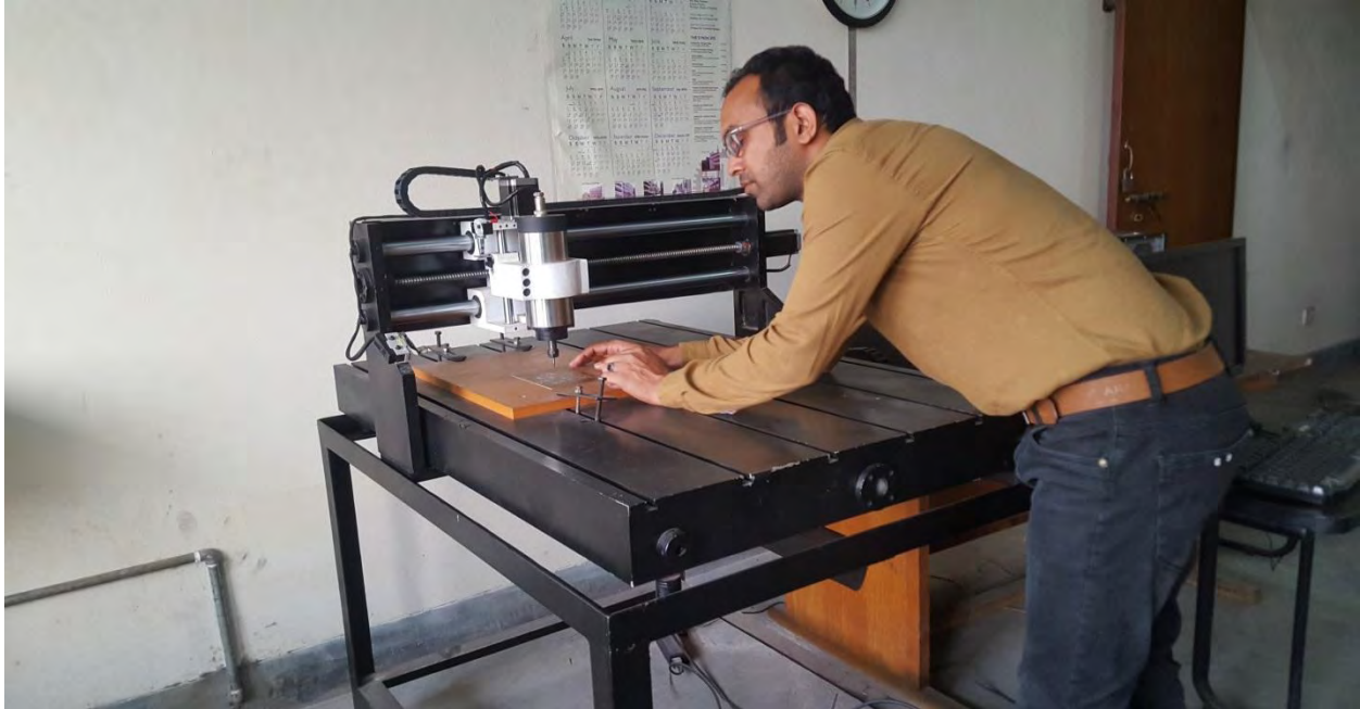
Figure 4.14: Monitoring PCB milling on CNC machine
