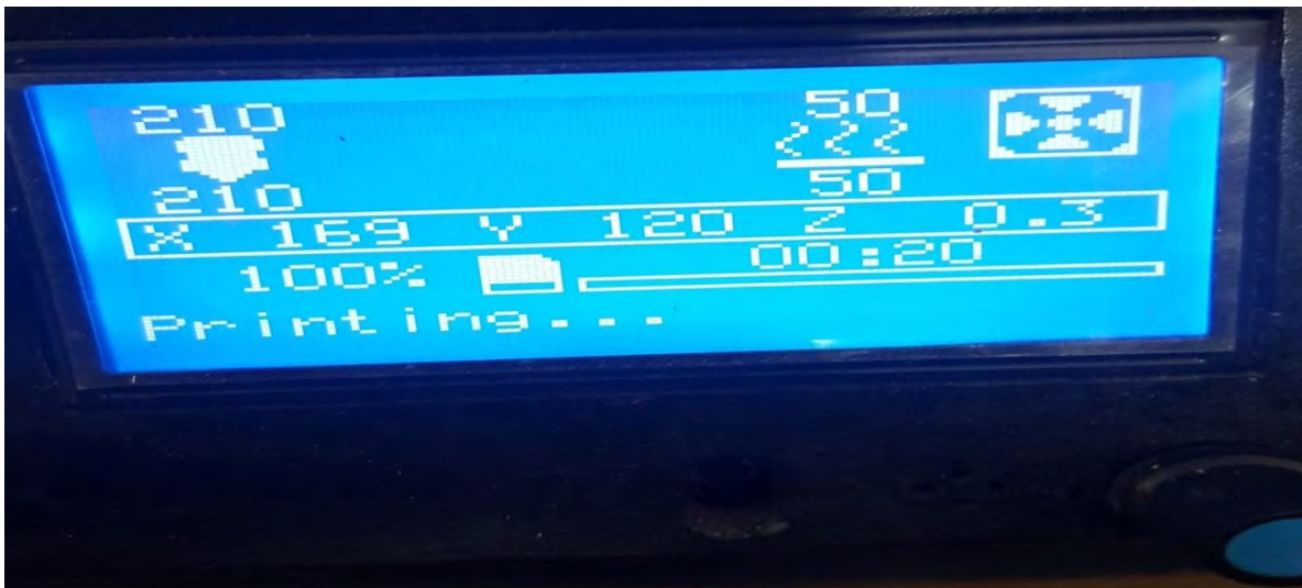
Figure 4.27: Printer Display when BOX printing, its time 20minutes.
