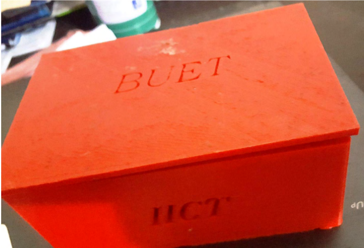
Figure 4.39: casing print using 3D printer
