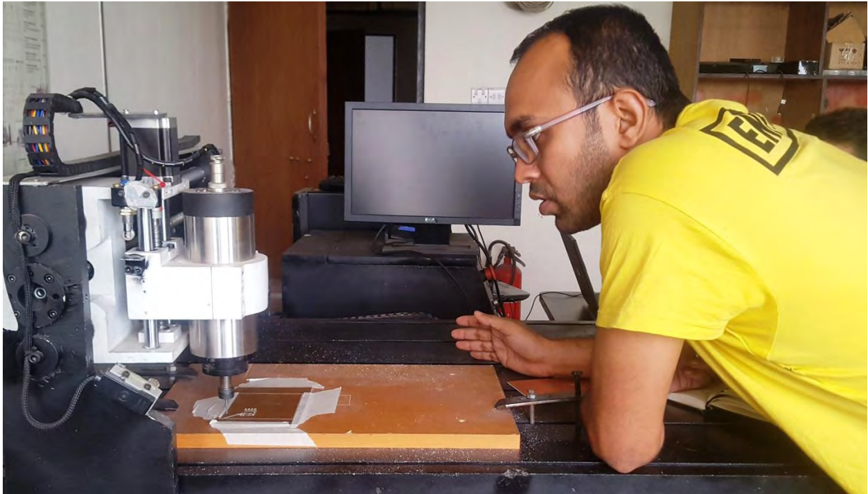
Figure 4.12: Drilling of PCB by CNC machine.
