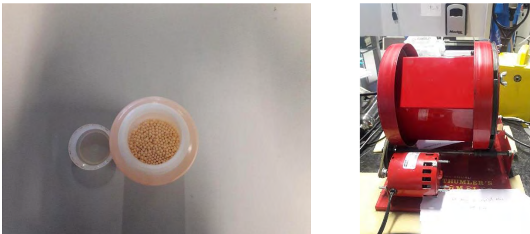
Figure 3-3: Milling pot with zirconia balls and ball mill setup. Adapted from [SPS lab UL]
