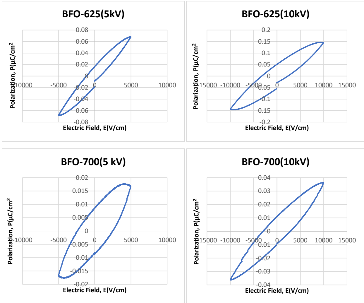
Figure 4-18: P-E curve for BFO-625 and BFO-700 at voltage 5 kV and 10 kV.
