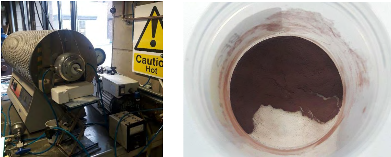
Figure 3-6: Furnace used for calcination and powders after calcination. Adapted from [CS lab UL]
