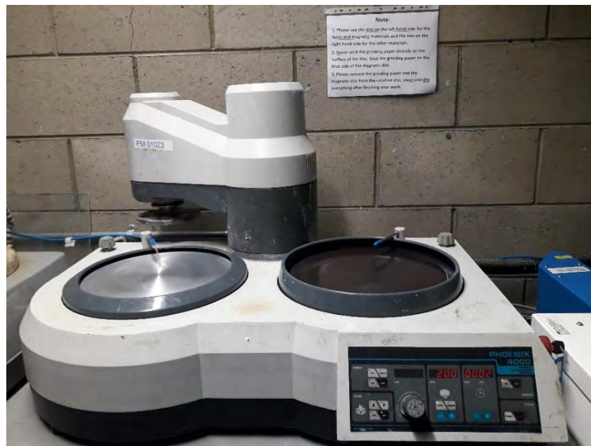
Figure 3-9: Polishing Machine(PM-01023). Adapted from[ CS lab UL]
