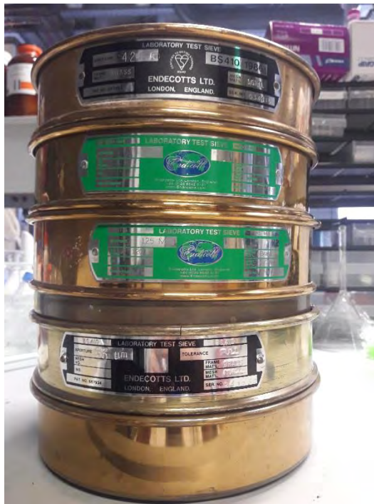
Figure 3-5: Laboratory Test sieve with different mesh size. Adapted from [CS lab UL]
