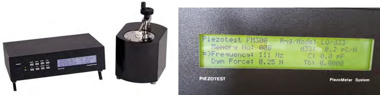
Figure 3-17: Piezo Meter and one of readings of the prepared BFO sample SPS sintered at 825 °C. Adapted from[ CS lab UL]
