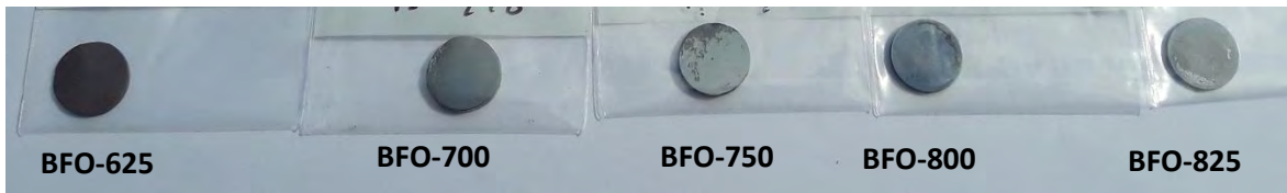
Figure 4-1: Prepared BFO pellets SPS sintered at 625, 700, 750, 800, 825°C respectively.
