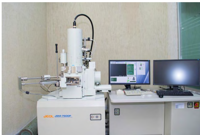
Figure 3-15: Field Emission Scanning Electron ( FESEM ). Adapted from [ GCE lab BUET]
