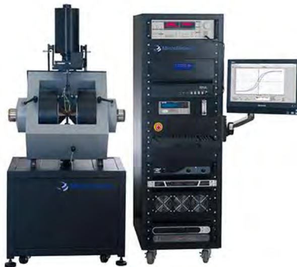
Figure 3-19: Vibrating Sample Magnetometer (VSM). Adapted from [ google image]
