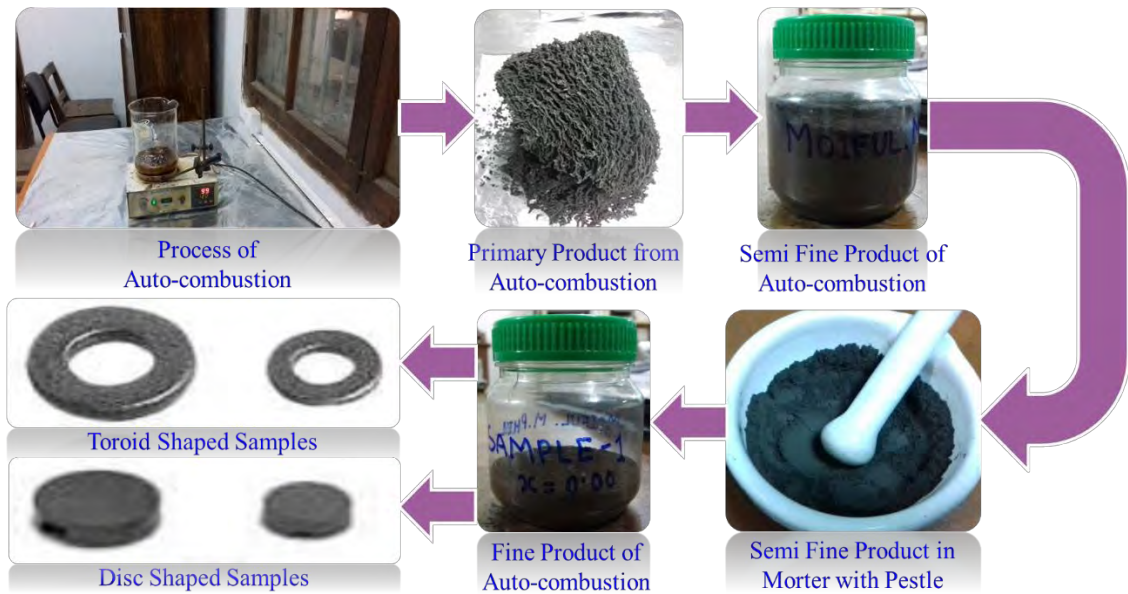
Fig. 3.3. Steps in preparation of present spinel ferrite samples.
