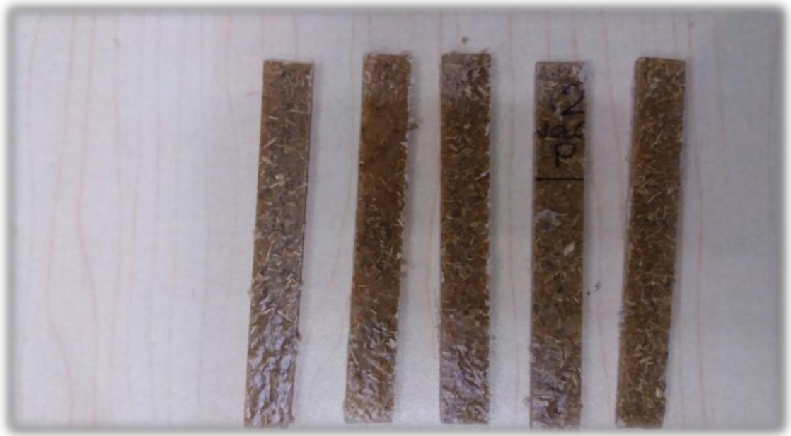
Figure 4.5.2.2: Tensile and flexural test specimen
