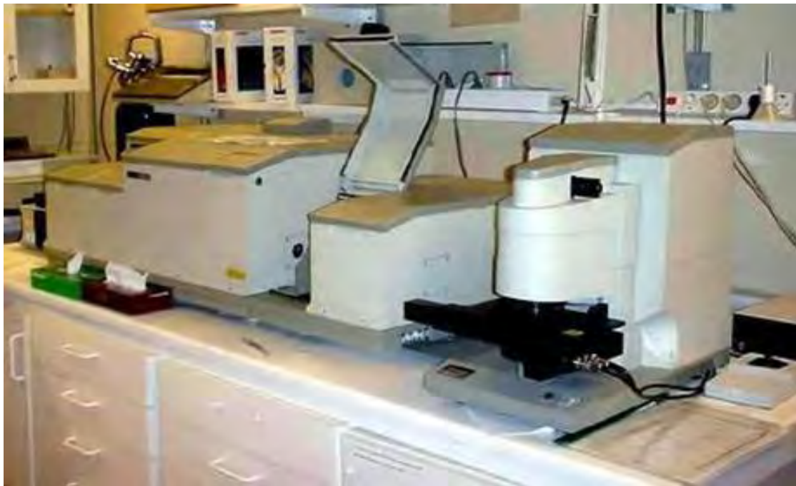
Fig.4.4.1: A photograph of an FT-IR spectrometer
