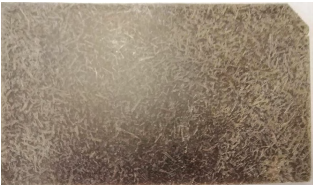
Fig 4.3.2.5 Composite prepared by compression molding
