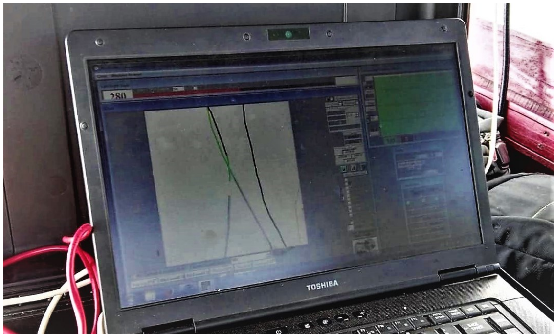
Photo 3.3: A portable computer with the hydro-pro software used for bathymetric survey.
