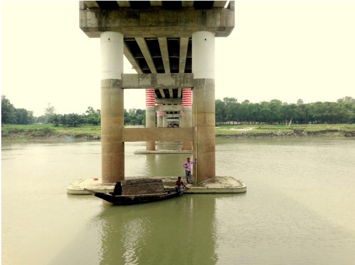
Photo 3.9: Setting up of the TBMs on a pier by the standard leveling instrument.
