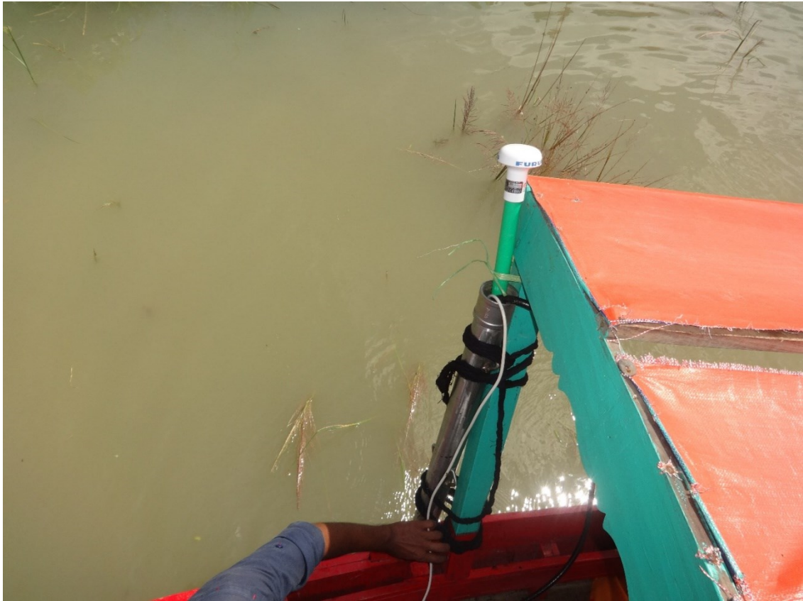
Photo 3.5: Transducer and DGPS antenna set up used for bathymetric data collection.
