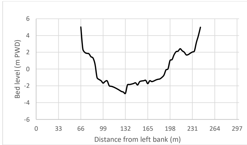
Figure B.46: Observed bed level on October 16 at bridge site.
